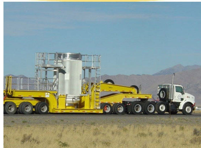
Large Cell Cask – NR SNF in transit from CPP-666 to NRF.
