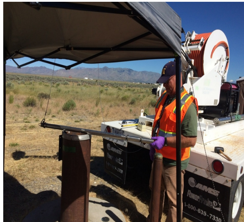
Filter-swab device containing granular activated carbon is used to remove PCE contamination in Westbay well tubing fluid.
