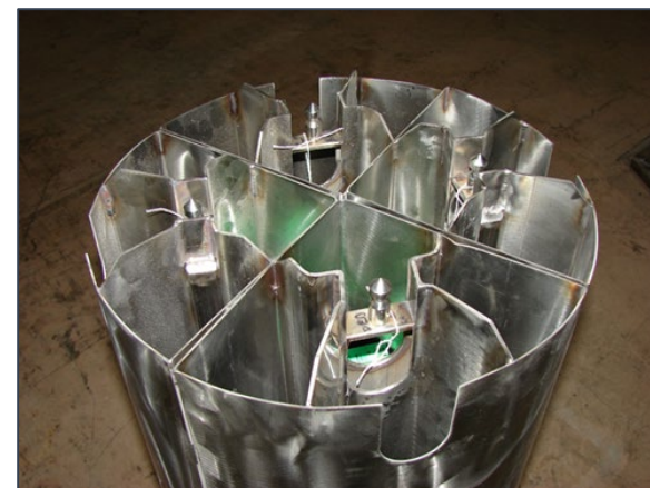
New four bucket storage design for placement of 16 ATR SNF elements into the CPP-603 storage canister – top view
