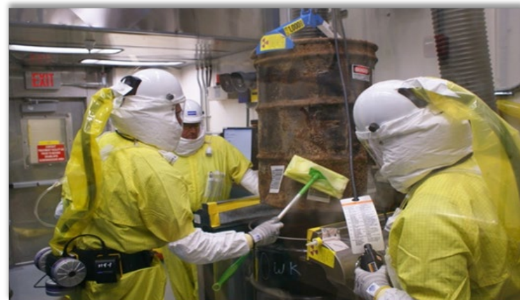
Overpacking CH-TRU waste
