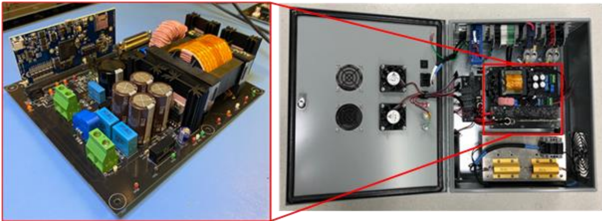
Custom-designed and built switch-mode power converter used to stress v-GaN diodes from AVOGY
