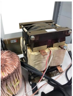
Multigap smoothing inductor 1mH, 1 kHz, six gaps
