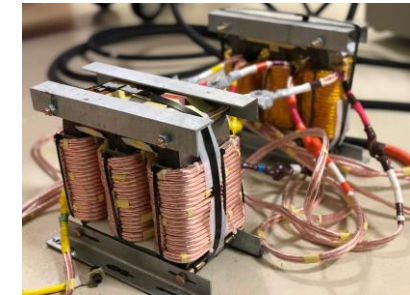
75 kVA Configuration Inverter Inductor Power Testing
