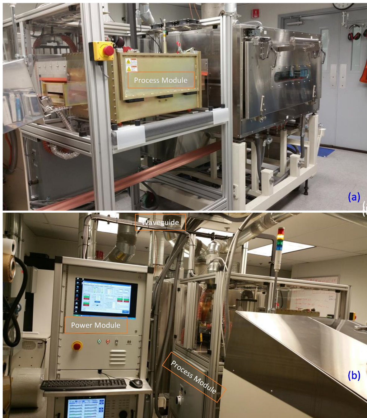
Figure IV- 268: (a) Digital image of the ADP Prototype installed at Navitas. The Process Module is in front while the Power Module is placed behind the Process Module, shown below it. (b) Digital image of the Power Module placed behind the Process Module delivering VFM power through the waveguide connecting both modules
