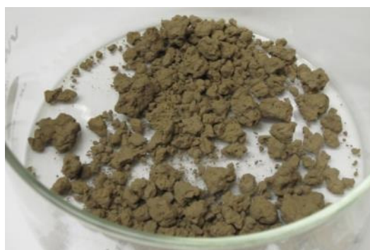
Figure IV- 225: 50 nm silicon coated with 10% w/w PFM (before milling); PSA of wet-blended Si-PFM/Nano-Si after milling
