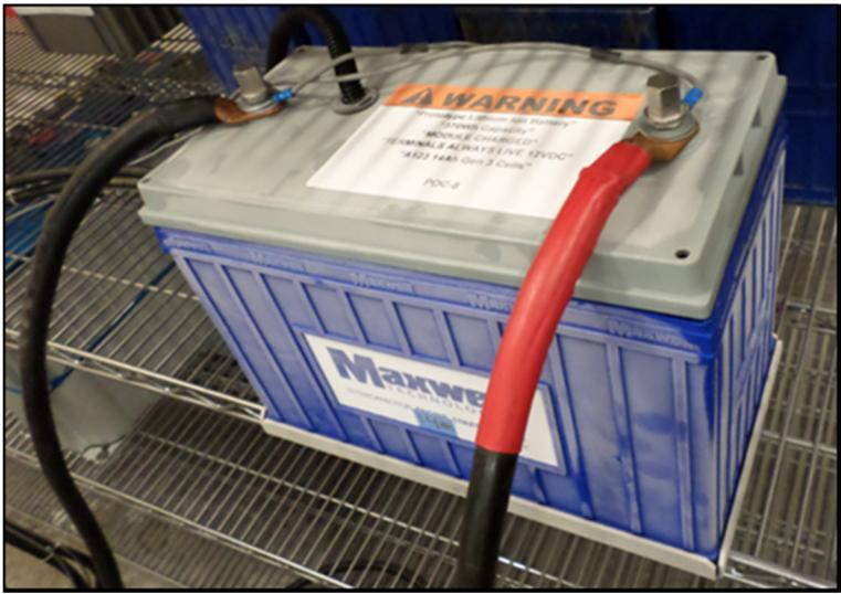
Figure II- 49: POC 9 built with the 20Ah Gen3 A123 cells
