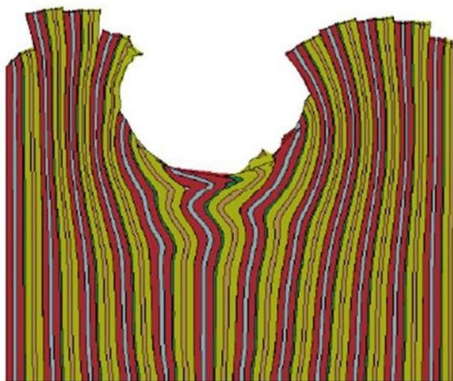
Figure III- 29: Sandwich model of a 12S1P battery crush test using a cylindrical impactor
