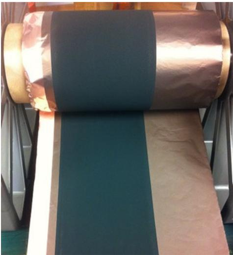
Figure II- 173: Slot-die coated low solvent anode with loading of 4 mAh/cm<sup>2</sup>
