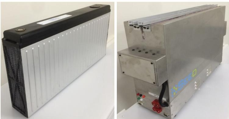
Figure II- 22: (left) Seo 1.8 kWh module. (right) Seo Single-Module Thermal Chamber (SMTC)
