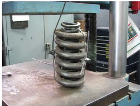
Middle truck corner springs compressed
