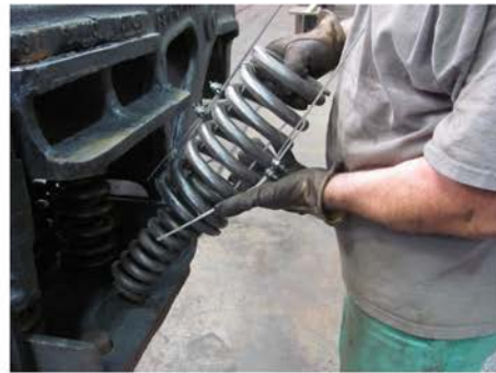
Middle truck center spring compressed
