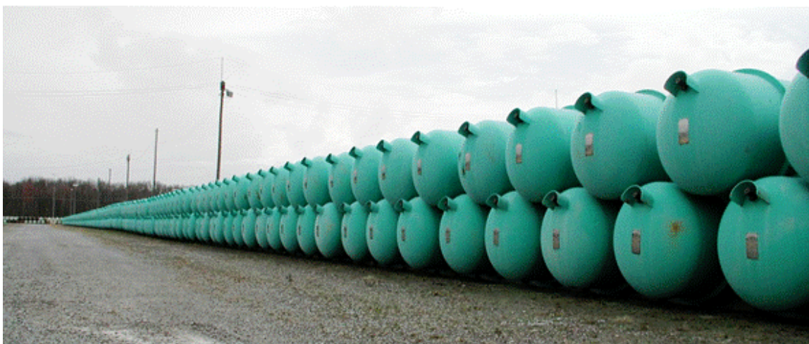
Figure 2-5 DUF 6 Cylinder Storage Yard (Source: BWXT 2016b)
