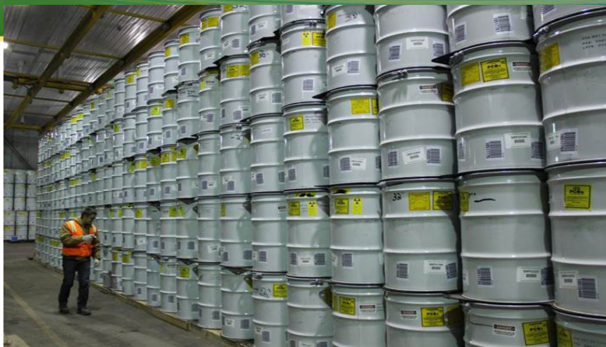
Left: 100-gallon product drums containing CH-TRU waste certified to ship to WIPP.
