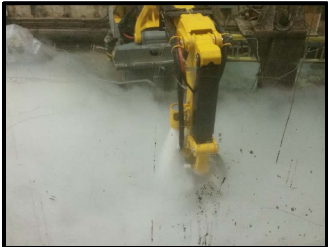
Above: CO 2 Test of New Brokk 400 prior to Operations
