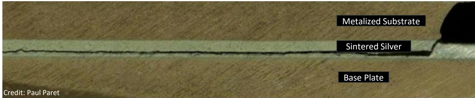
Crack Propagation in Pressure-Assisted (30- 40 MPa) Sintered Silver
