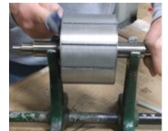
Rotor with Magnets
