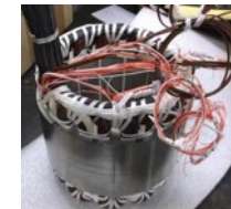
Stator with Winding
