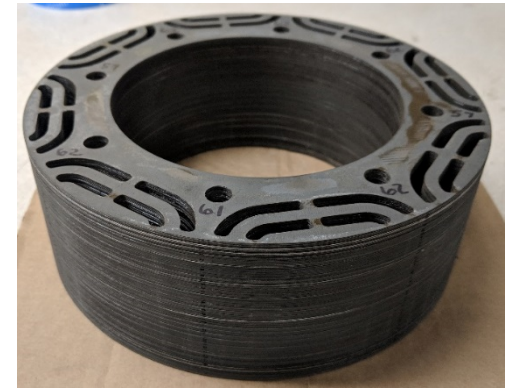
Dual Phase Rotor Laminates
