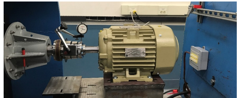
Motor on test stand
