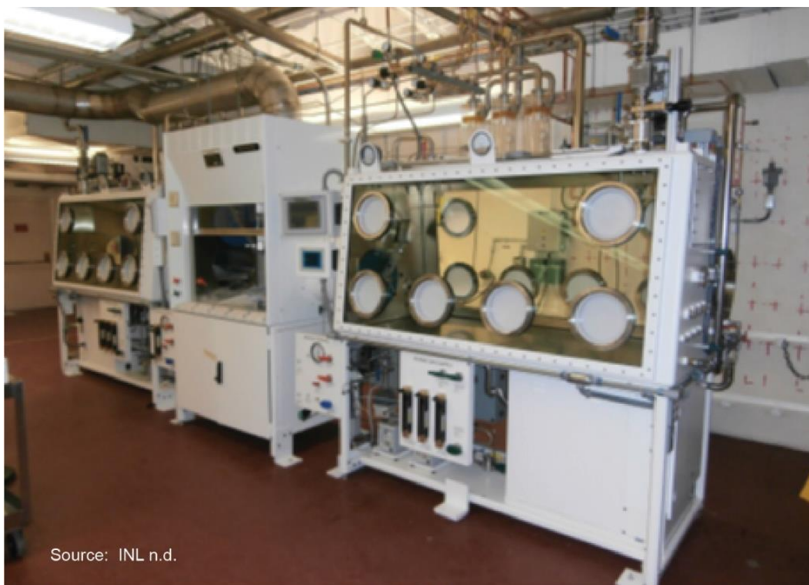
Figure S–6. Representative Glovebox
