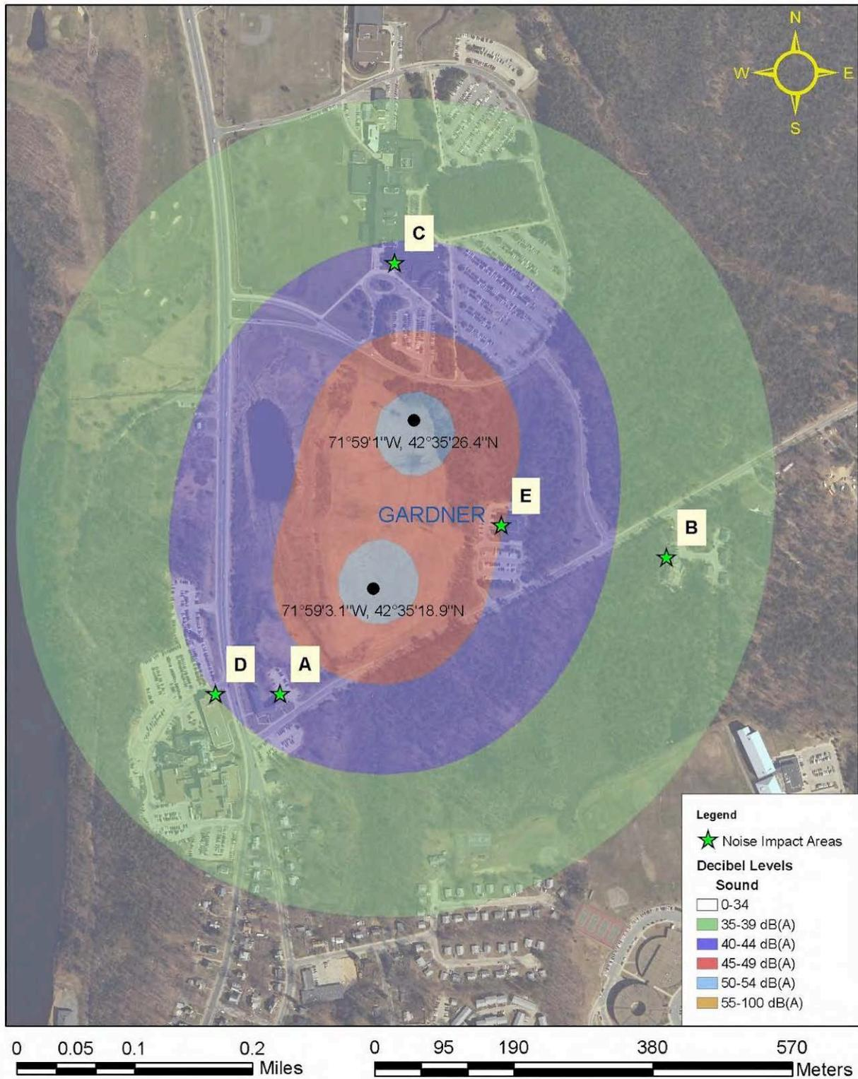
**Figure 3:** Orthophotograph with an overlay of estimated decibel levels at a wind speed of 8 m/s from proposed wind turbine installation in Gardner. *Orthophotograph courtesy of MassGIS.*
