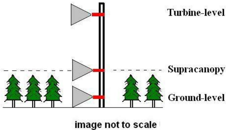
**Figure 2. Schematic of Meteorological Tower microphone array**
