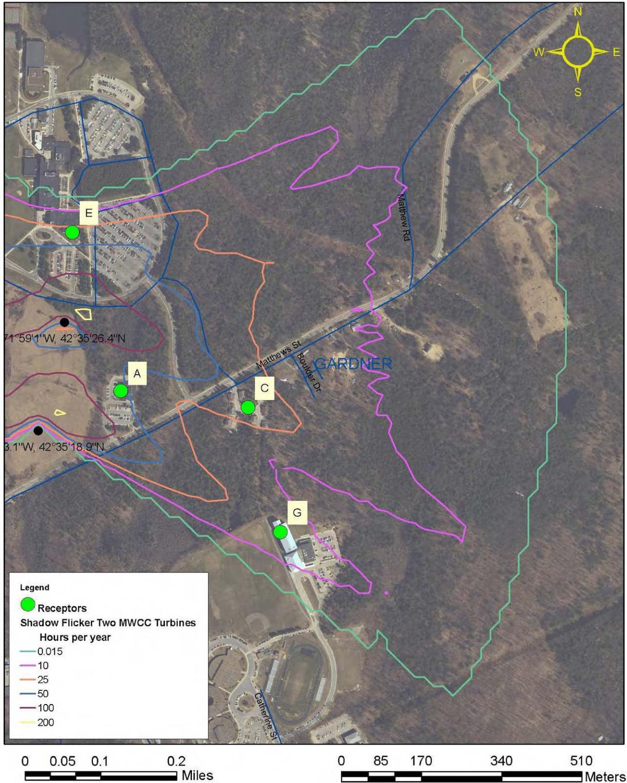
**Figure 4:** This figure shows the shadow flicker isolines to the east of the turbines in hours/year. Regions inside the purple line feature expected values for shadow flicker duration of at least 10 hour per year. There are several residences in the area that are expected to have between 0.015-25 hours of shadow flicker.
