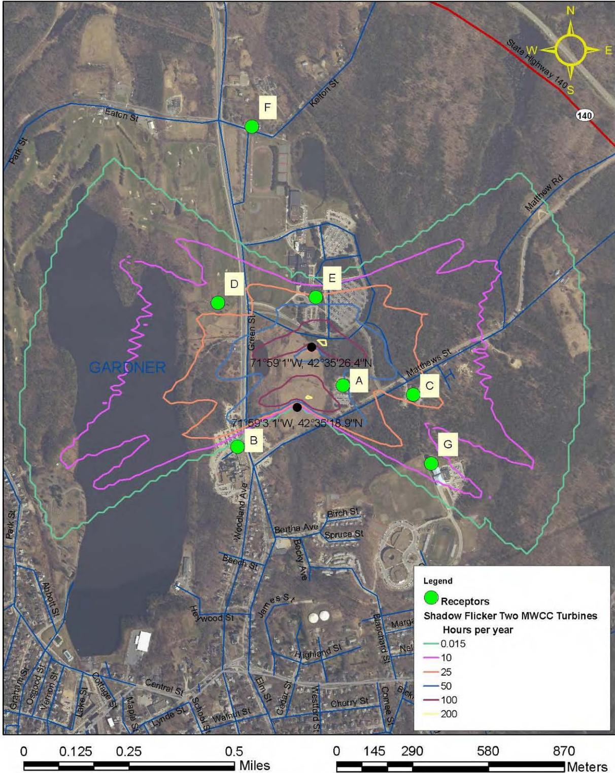
**Figure 3:** This figure shows an orthophotograph of MWCC turbine site with isolines showing estimated shadow flicker in hours/year. Regions inside the purple line feature expected values for shadow flicker duration of at least 10 hour per year. Receptor A (Courthouse) shown on the map above, features an expected value of 53 hours and 7 minutes (value found in **Table 4**).
