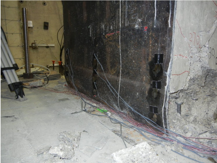
Out-of plane specimen ~peak load
