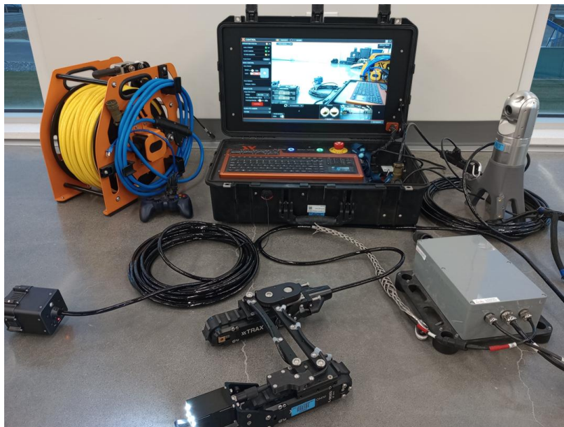
Figure 7. Nexxis system components and Juicebox controller.
