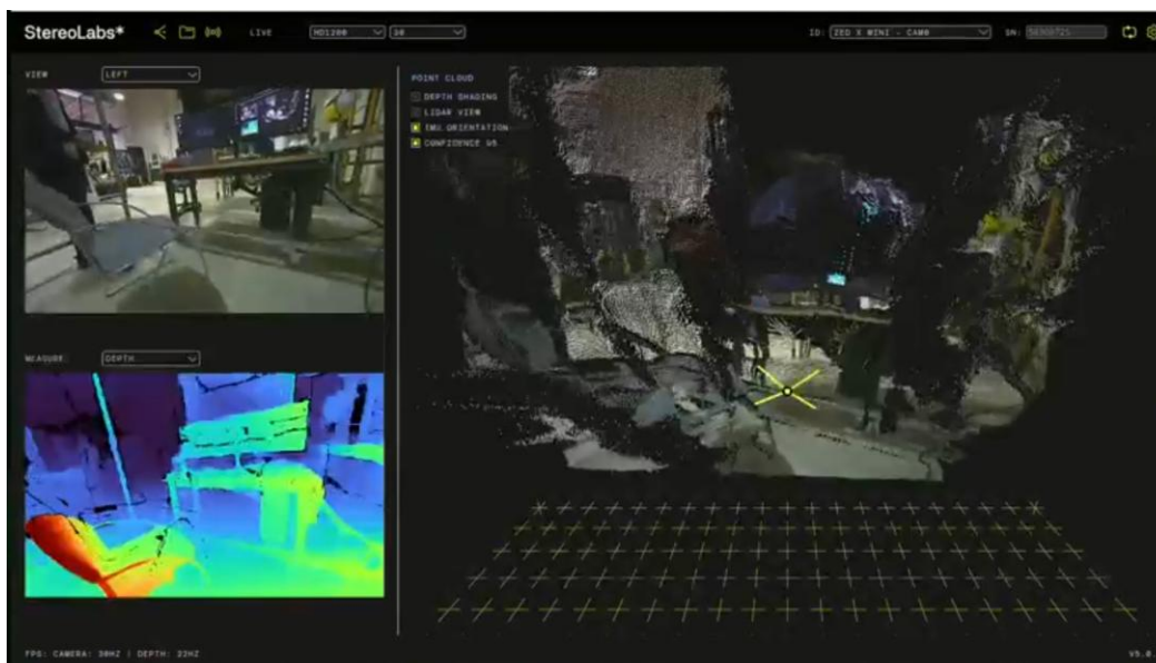
Figure 23. Live inspection scene captured by the ZED X Mini stereo camera at the robot's end-effector. The StereoLabs interface shows (left) the RGB view and color depth map, and (right) the live 3D point cloud with IMU orientation overlay. This data is streamed in real time to the ROS 2 planning stack.
