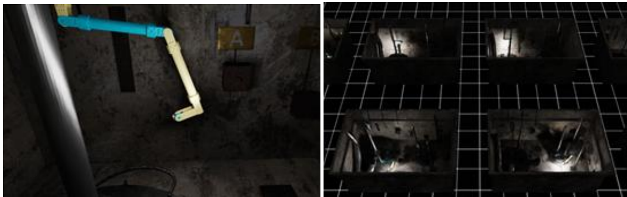
Figure 13. (left) Robotic arm tracked via PTZ camera with RTX path-traced lighting and (right) multi-environment simulation with randomized initial configurations.
