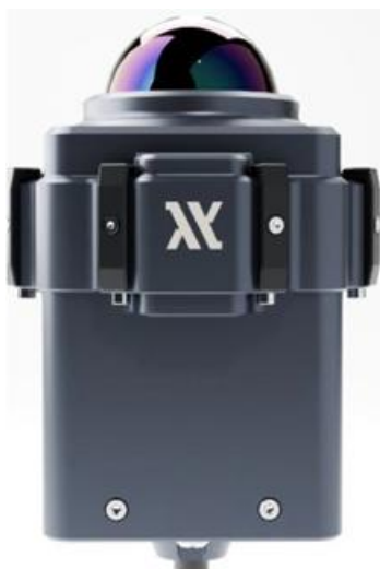
Figure 10. Nexxis Argus, custom-designed for s 4-in. view port.
