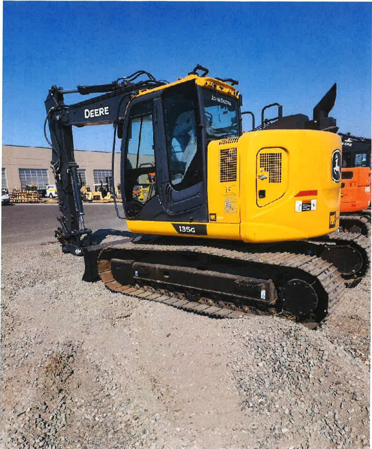
Figure 10 – Steel Tracked Excavator
