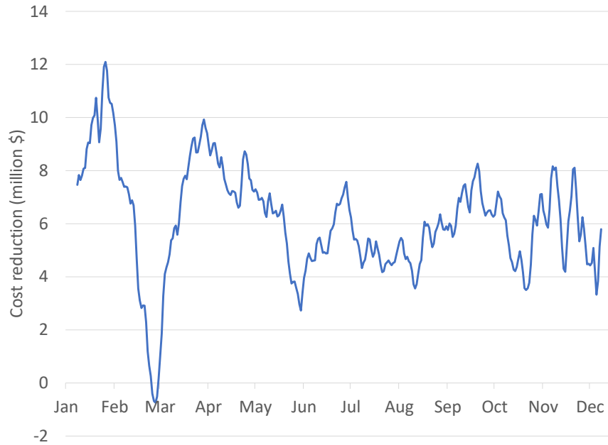
Figure 52. Daily cost reduction from hydropower flexibility
