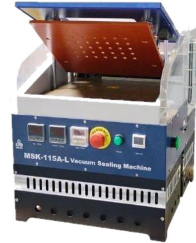
Recently acquired vacuum sealing machine to produce prototype VIPs using different core materials
