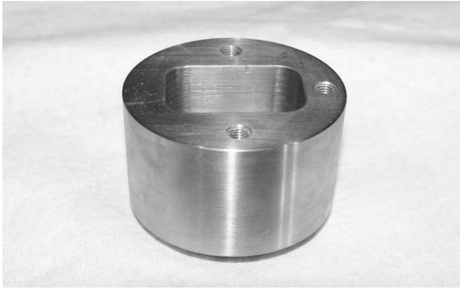
Figure 62. Custom in situ TPS sample holder. 154
