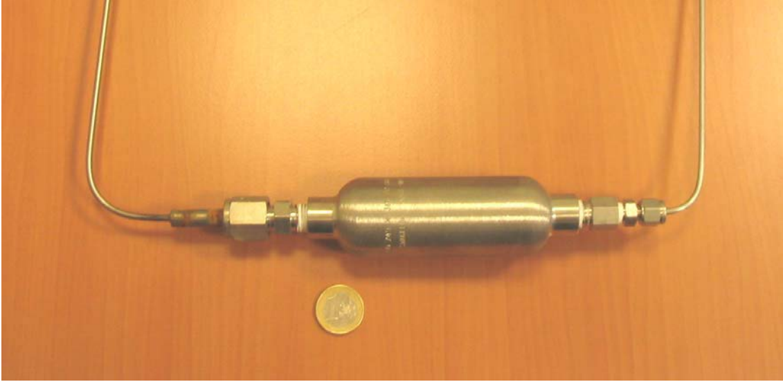
Figure 43. View of the buffer tank with the hydrogen connection (left) and thermocouple inlet (right). 194
