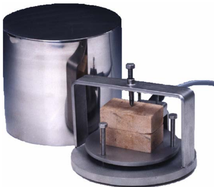
Figure 25. An image of an example TPS measurement setup. 146
