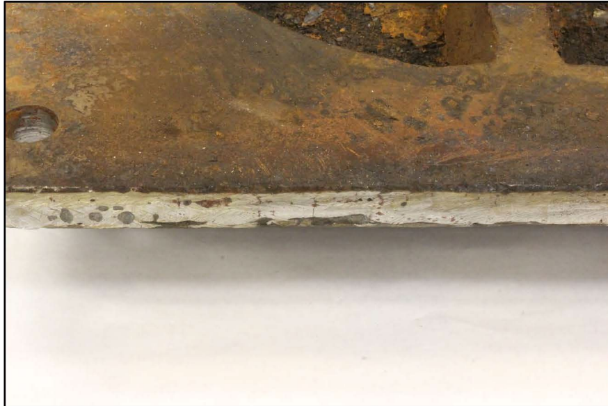
Figure 2. Image showing a cluster of cracks identified as Region A. A number of individual vertical cracks were evident on the cut and ground surface.
