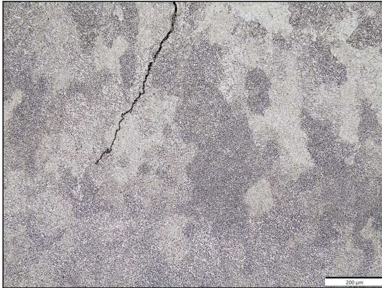
Figure 21. Metallographic image showing the typical weld zone microstructure. (2% Nital etch, 100X)
