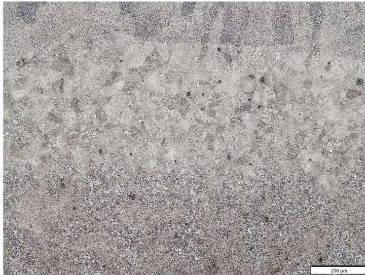
Figure 19. Metallographic image showing the typical heat affected zone microstructure of the cast steel plate adjacent to the weld. (2% Nital etch, 100X)
