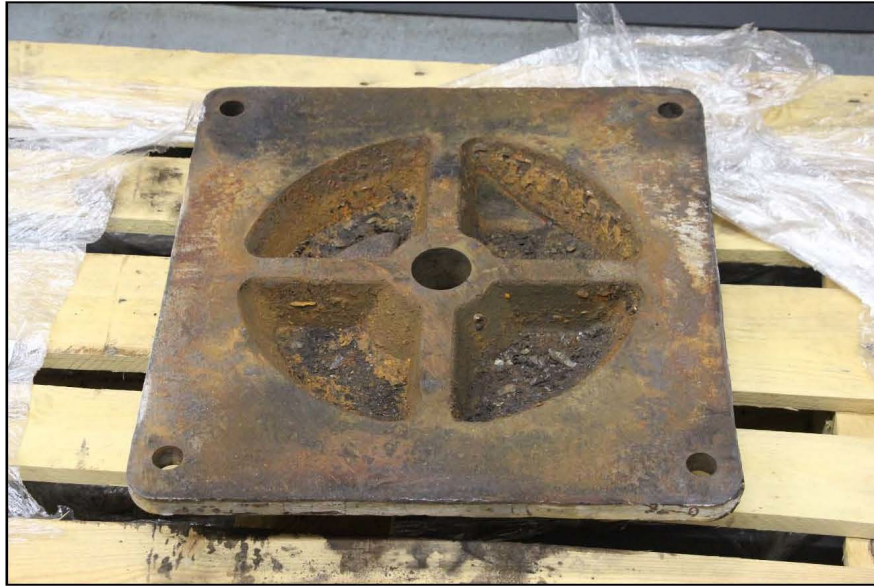
Figure 1. Photograph showing the submitted center plate. The ground weld edge that exhibited cracks is toward the bottom in this image.
