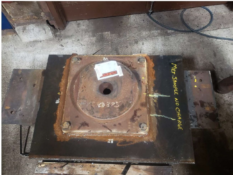
Figure 1: Image of Trispan Test Piece showing two ( 2 ) crack indications on the BR side of the sample
