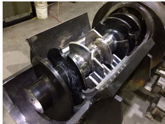
Re-designed auger-grinder.
