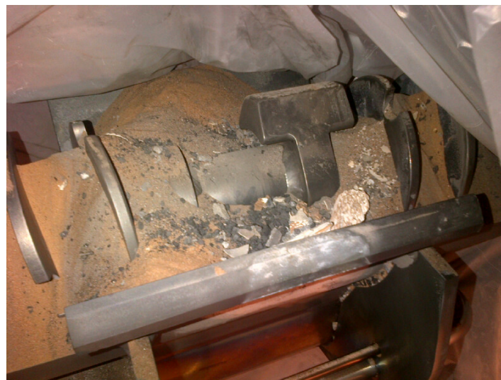
Auger-grinder has been redesigned to better handle large rocks.
