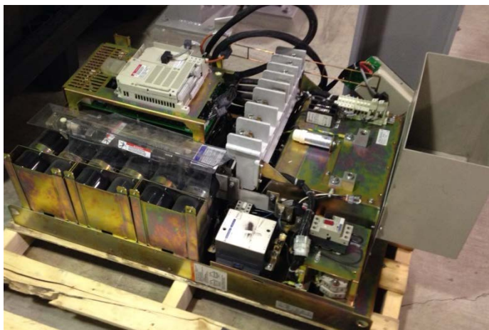
Below: Obsolete VFD Removed from Ventilation System
