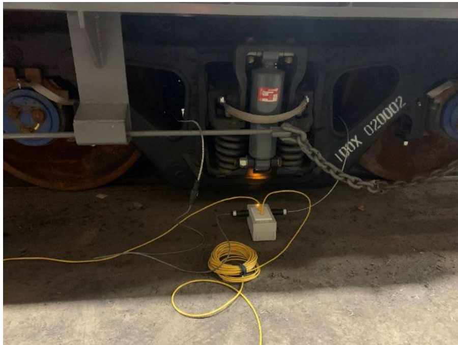
Figure B4. Brake Force Measurement System (B-end L1, L2 Force Sensors)
