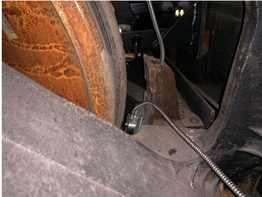
Figure B5. Example Force Sensor Location
