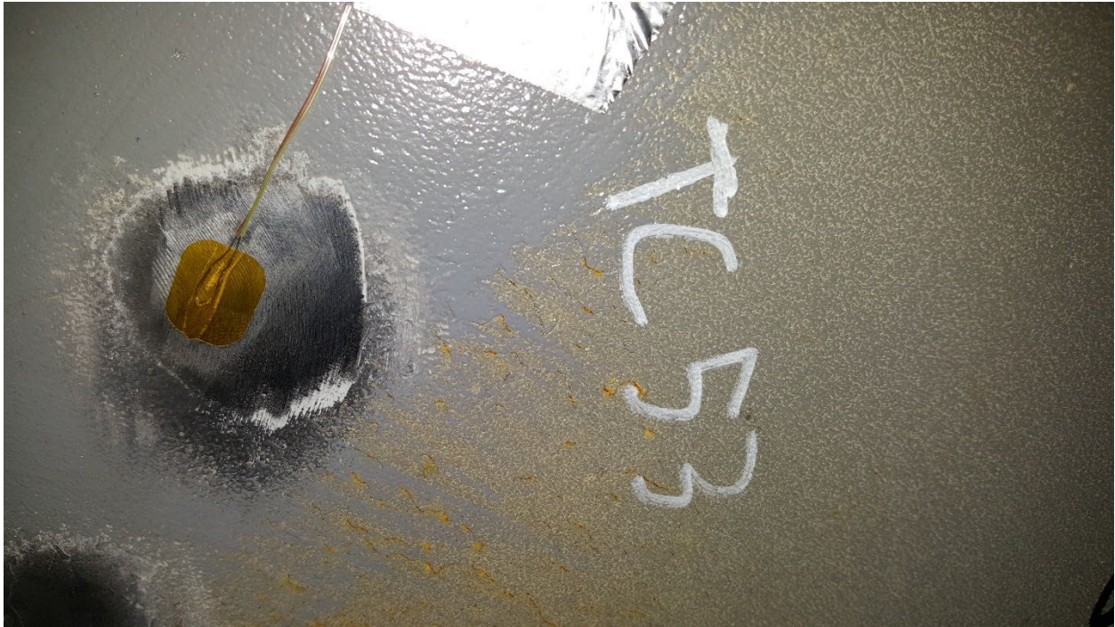
Figure C57. TC53 Laterally and Longitudinally Centered on top of Deck Plate Forward of A-End Body Bolster
