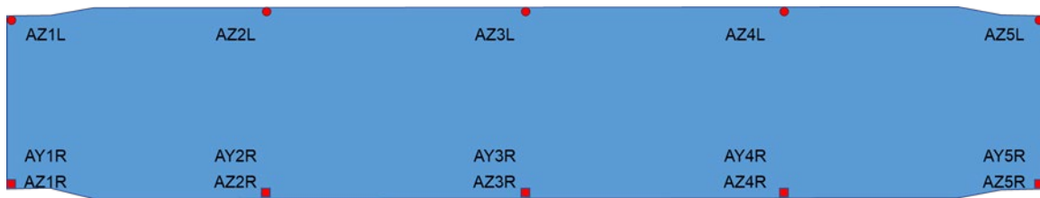
Figure 30. Distribution of Accelerometers during the Buffer Railcar Modal Test
