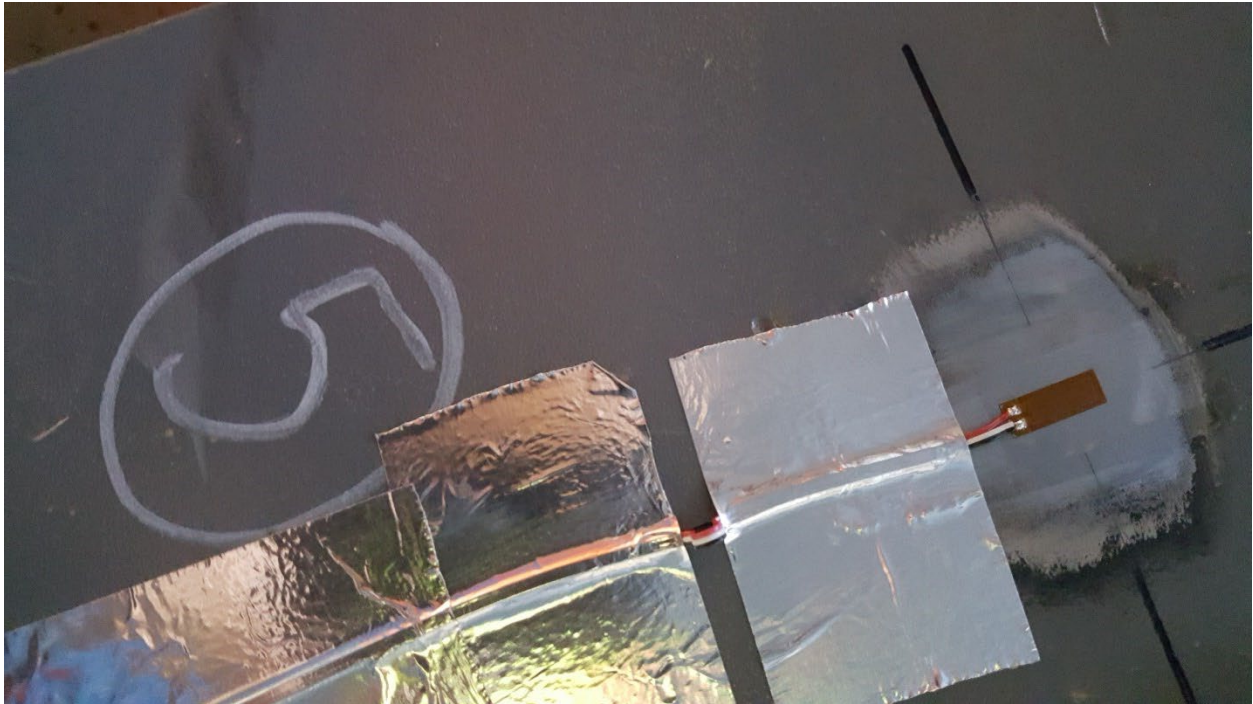
Figure C9. SGBF5 RH Edge of Bottom Flange of Center Sill, Aft of A-end Body Bolster
