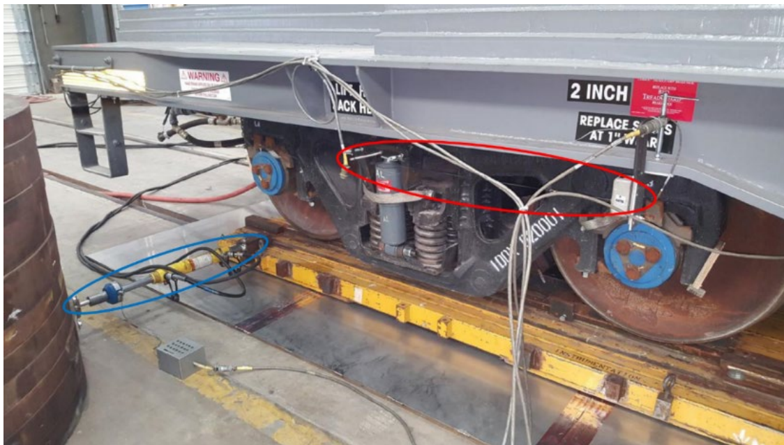
Figure 25. Buffer Railcar Positioned on Air Bearing Table
