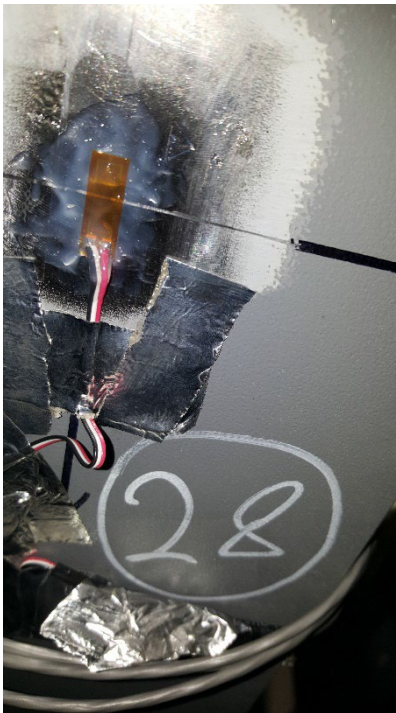
Figure C32. SGBF28 Center of Bottom Flange of RH Side Sill, at Longitudinal Center of Car
