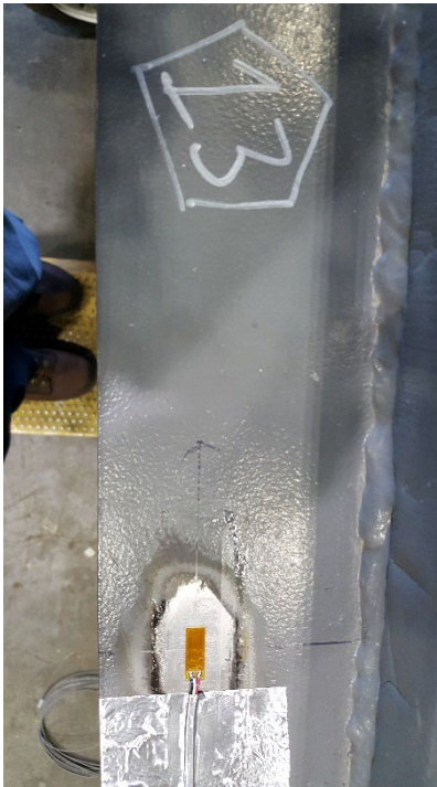
Figure C17. SGDP13 LH Edge of Deck Plate, Forward of Cross Bearer 7
