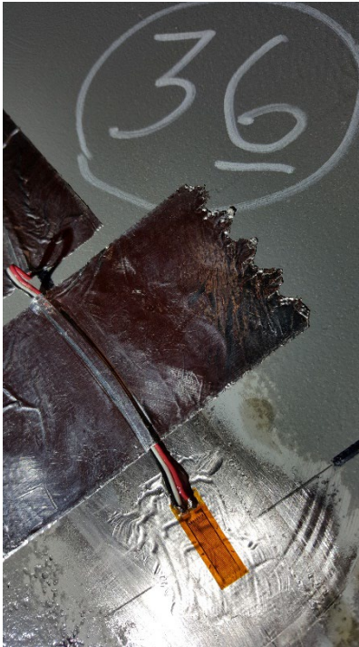
Figure C40. SGBF36 LH Edge of Bottom Flange of Center Sill, Aft of Cross Bearer 2
