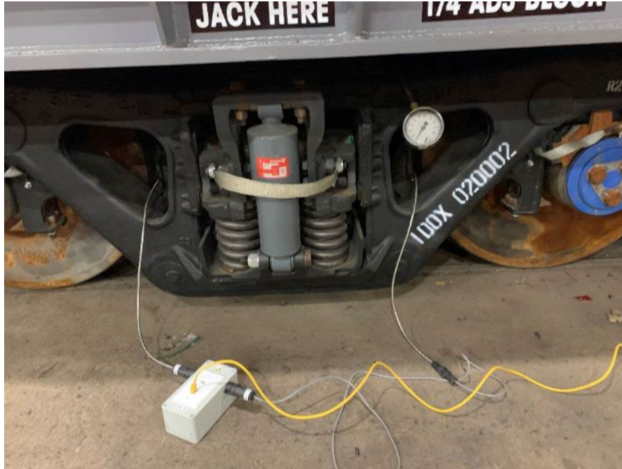
Figure B12. Brake Cylinder Gauge Location (B-end, Right Side)
