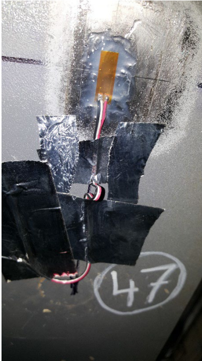
Figure C51. SGBF47 Center of Bottom Flange of RH Side Sill, Forward of Cross Bearer 1
