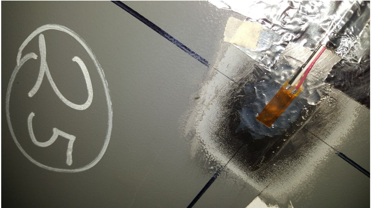
Figure C29. SGBF25 RH Edge of Bottom Flange of Center Sill, at Longitudinal Center of Car
