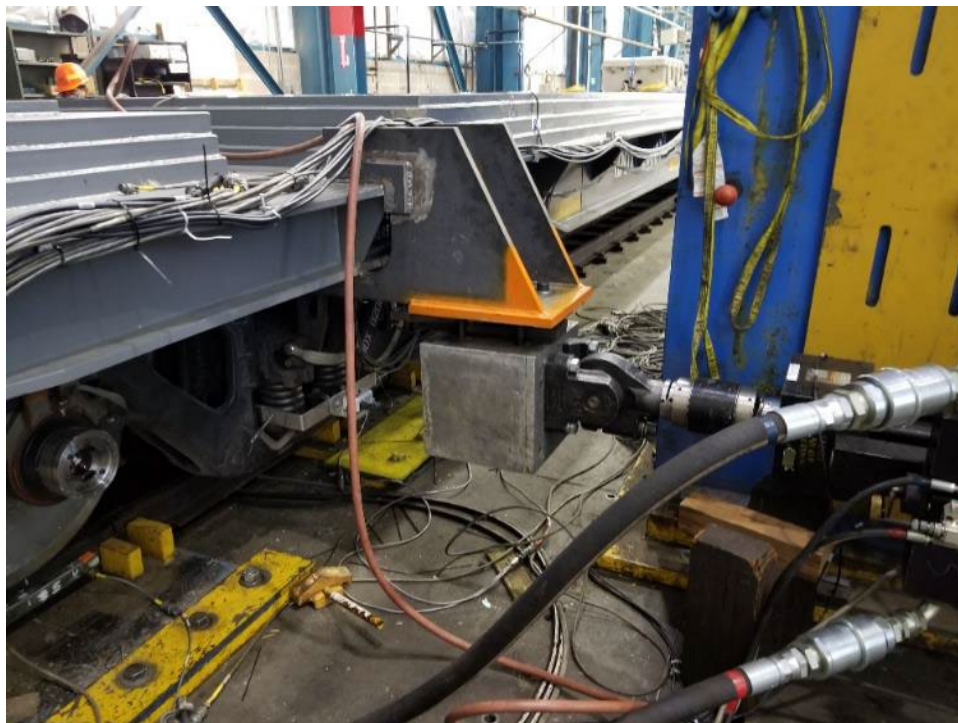
Figure 19. Buffer Railcar Ready for Lateral Force Test
