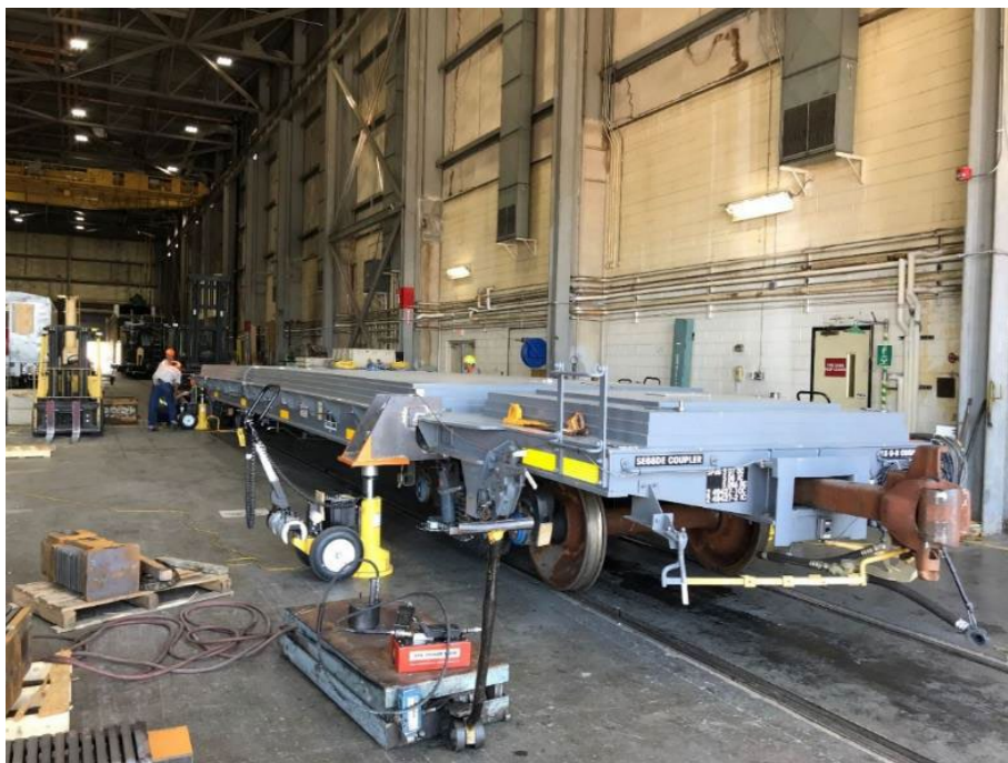
Figure 42. The End of the Railcar Supported by Four Pneumatic Jacks during the Twist Test
