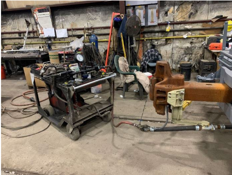
Figure B10. Single Car Air Brake Test Device
