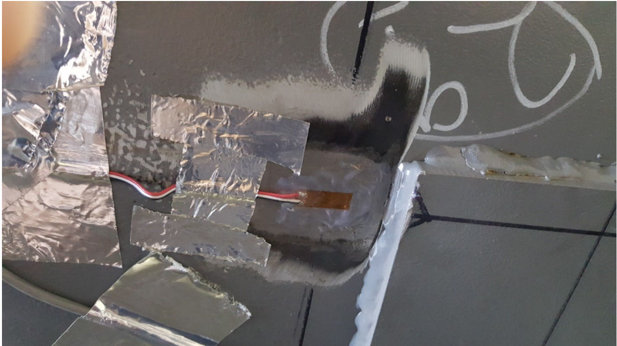
Figure C33. SGBF29 Center of Bottom Flange of LH Side Sill, at Longitudinal Center of Car
