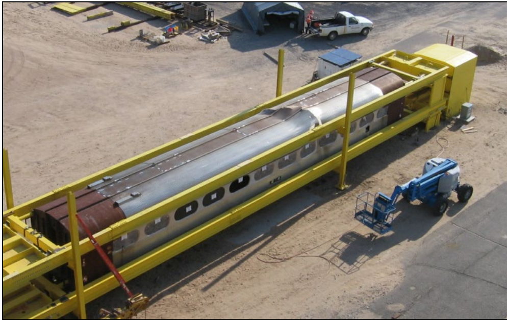
Figure 73. 2 1/2 Million-Pound Squeeze Test Fixture with Passenger Car Taken to Structural Failure
