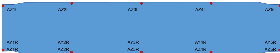
Figure 71. Locations of Modal Accelerometers
