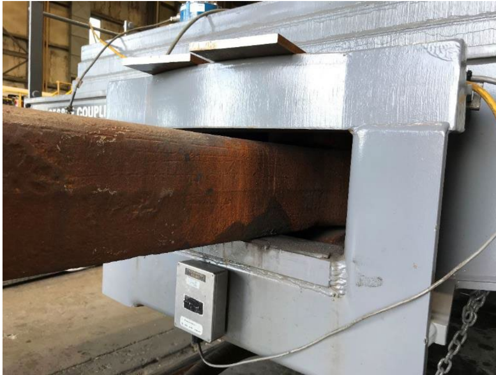
Figure 40. Coupler Carrier Plate after the Coupler Vertical Load Test
