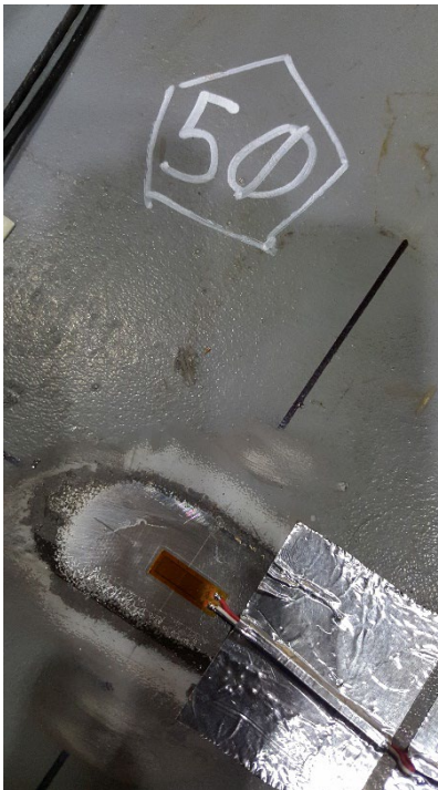
Figure C54. SGDP50 Top of Deck Plate, Longitudinally Centered over A-End Body Bolster, above RH Edge of Center Sill
