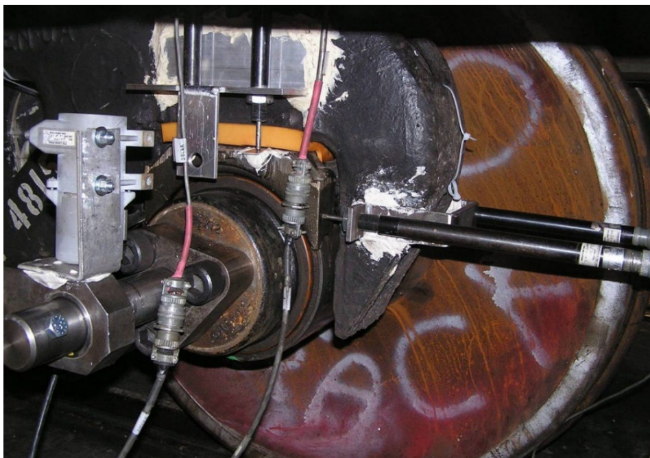
Figure 69. Inter-Axle Stiffness Test Setup Showing LVDTs for Measuring Pitching and Yawing of Bearing Adaptor
