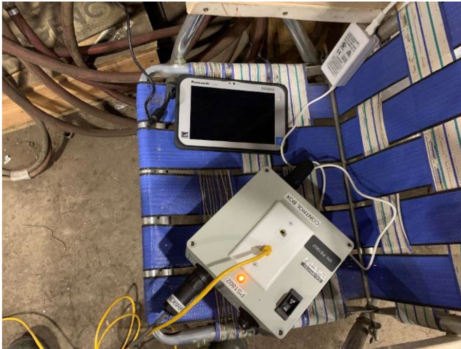
Figure B2. Brake Force Measurement System (Control Box and Readout Tablet)
