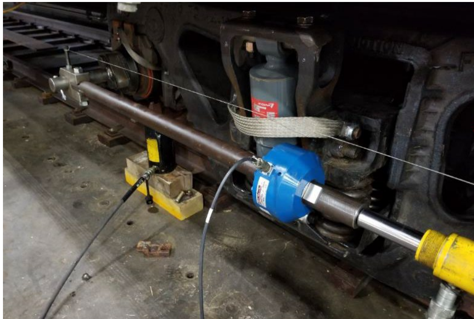
Figure 27. Buffer Railcar Interaxle Test Actuator and Load Cell
