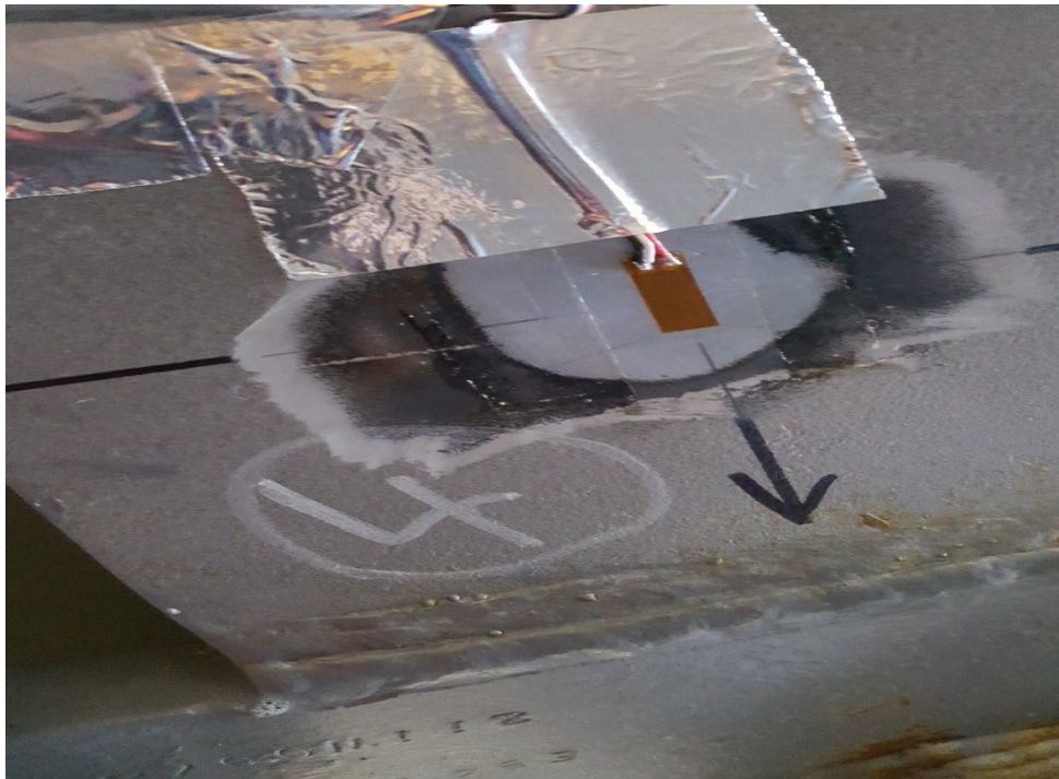
Figure C8. SGBF4 Rear of Bottom Flange of A-end Body Bolster near Center Sill, RH Side
