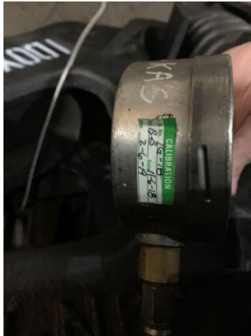
Figure B13. Brake Cylinder Gauge Calibration Information
