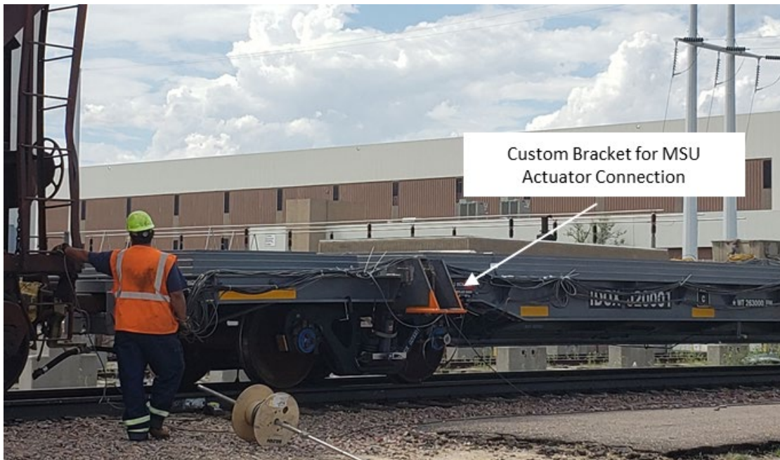
Figure 11. Brackets for Vertical and Lateral Actuators
