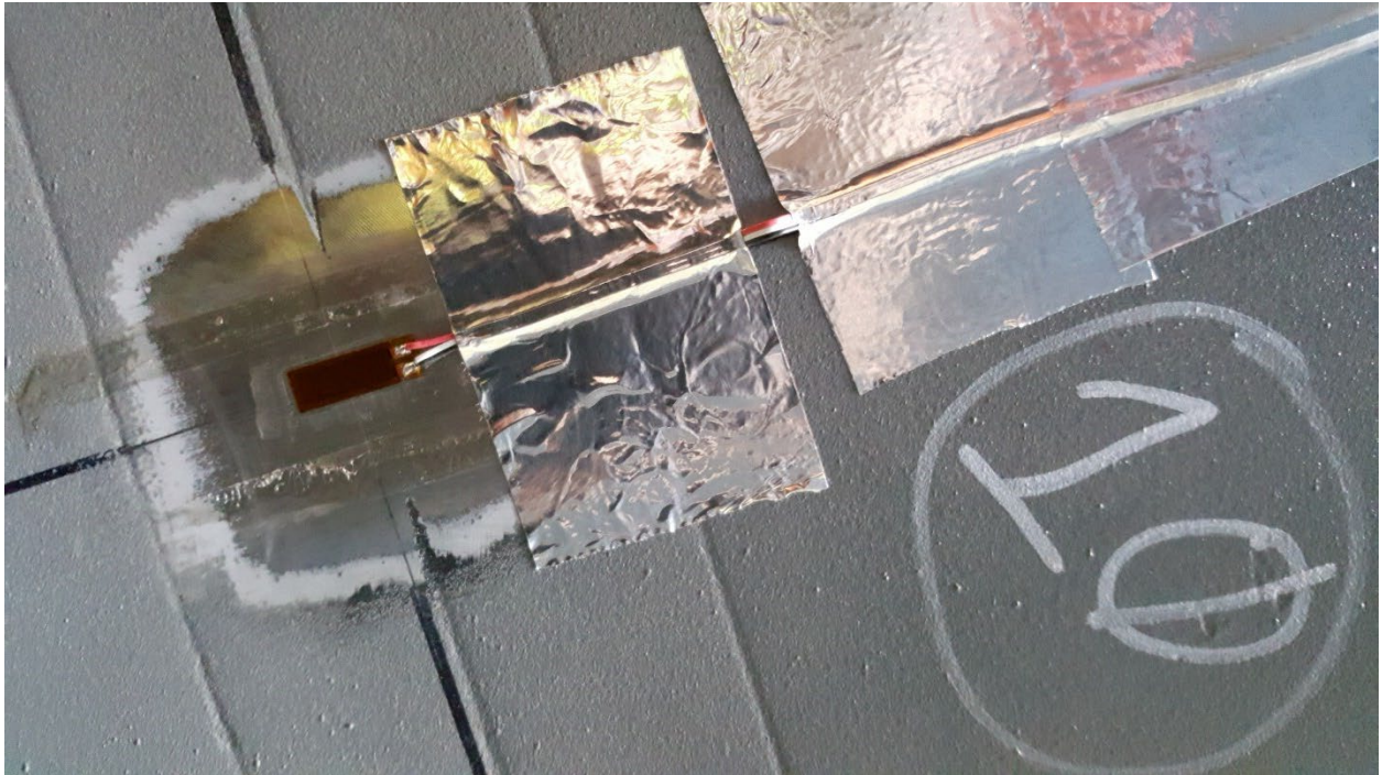
Figure C14. SGBF10 LH Edge of Bottom Flange of Center Sill, Forward of Cross Bearer 7
