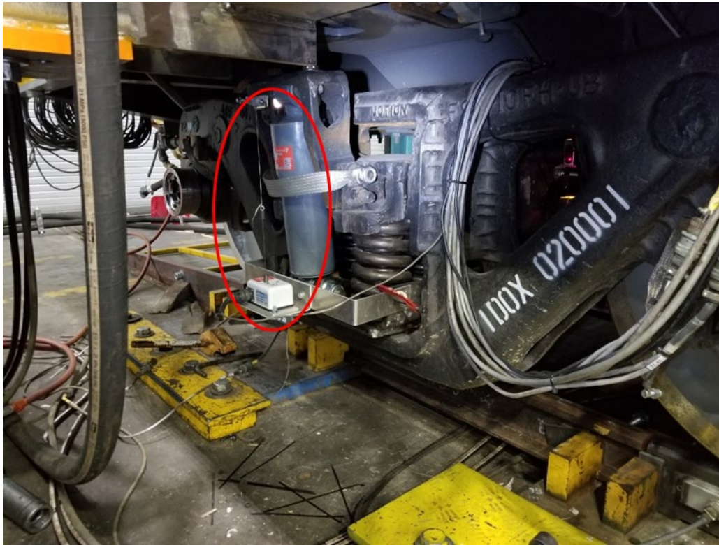
Figure 13. String Potentiometer for Measuring Spring Vertical Displacement (Damper Installed)
