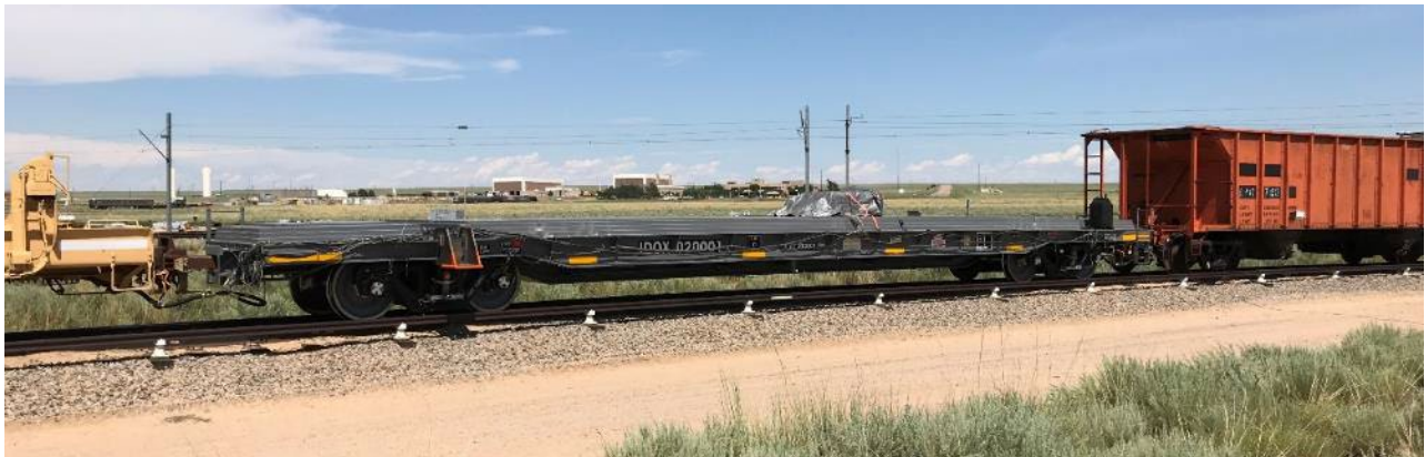
Figure 1. Buffer Railcar during Static Testing
