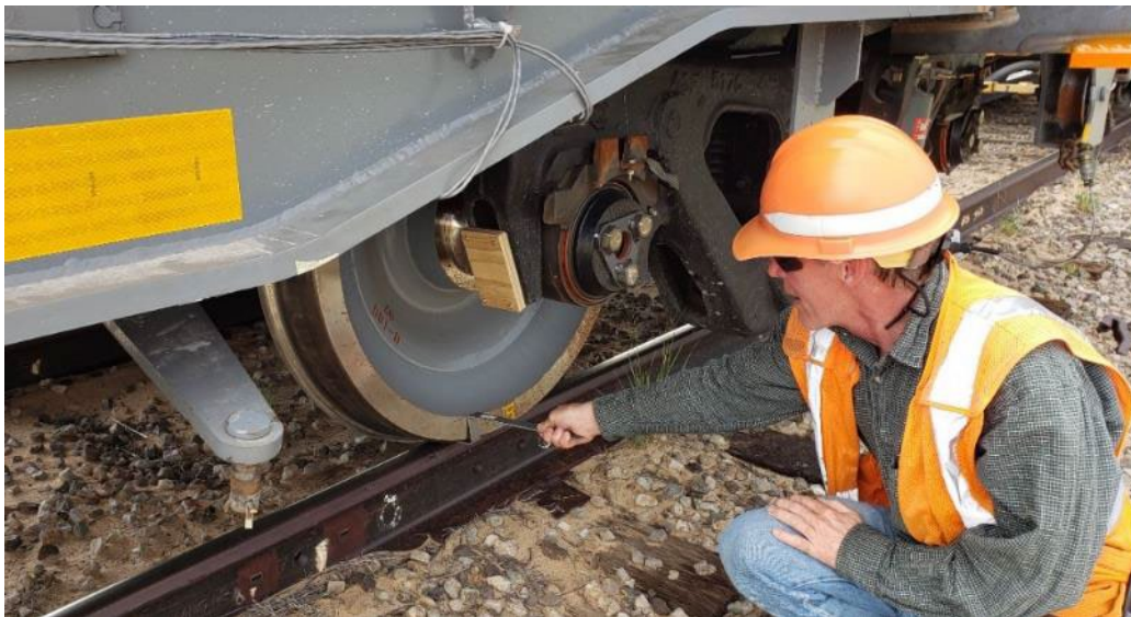
Figure 36. Checking Clearance during the Static Curve Stability Test
