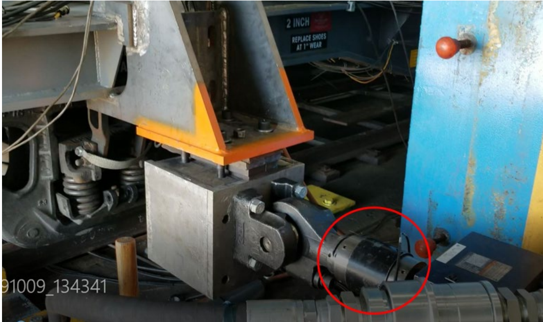
Figure 20. Load Cell for Lateral Force Measurements
