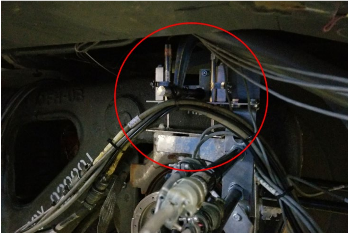
Figure 15. LVDTs for Measuring Pad Vertical Displacements
