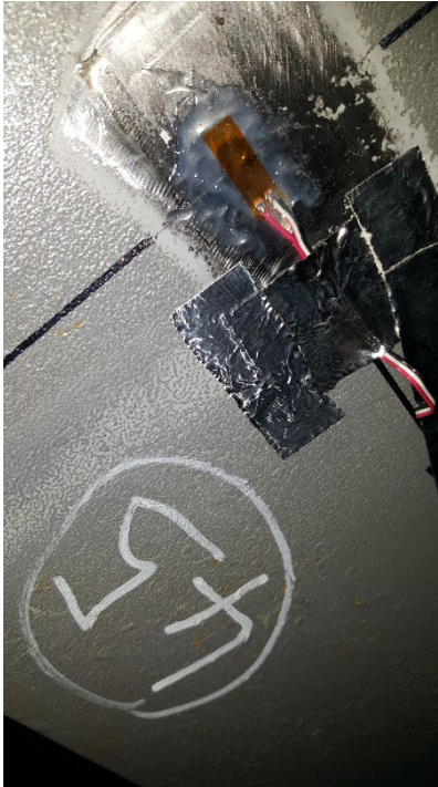
Figure C49. SGBF45 LH edge of Bottom Flange of Center Sill, Forward of B-end Body Bolster
