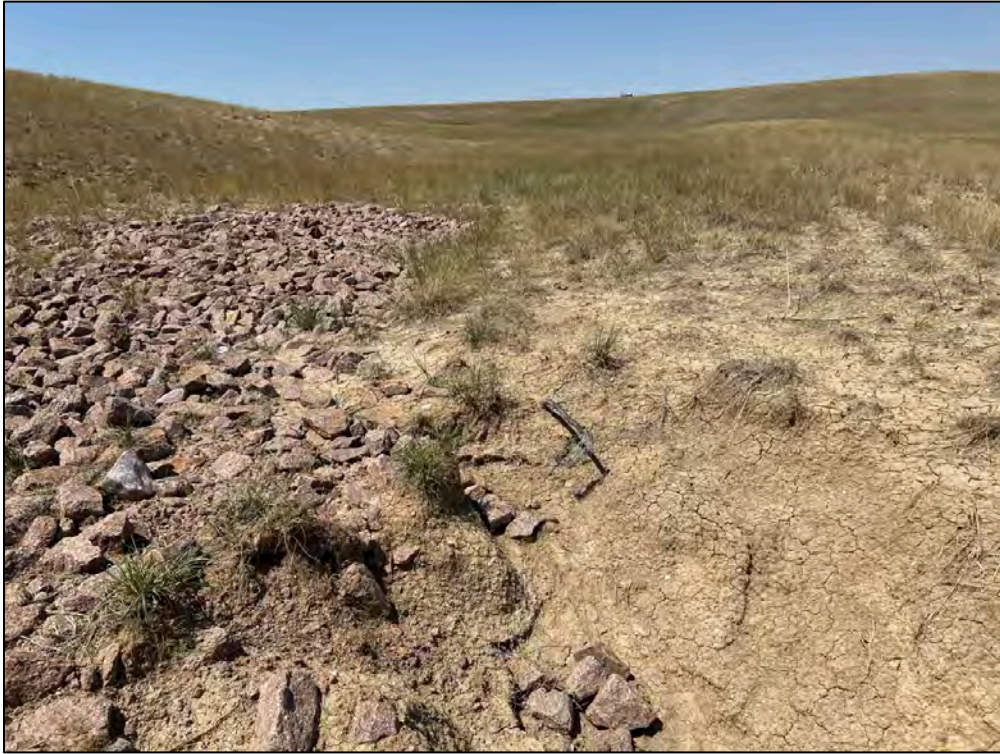
PL-9. Exposed Wire at Top of Erosion Gully
