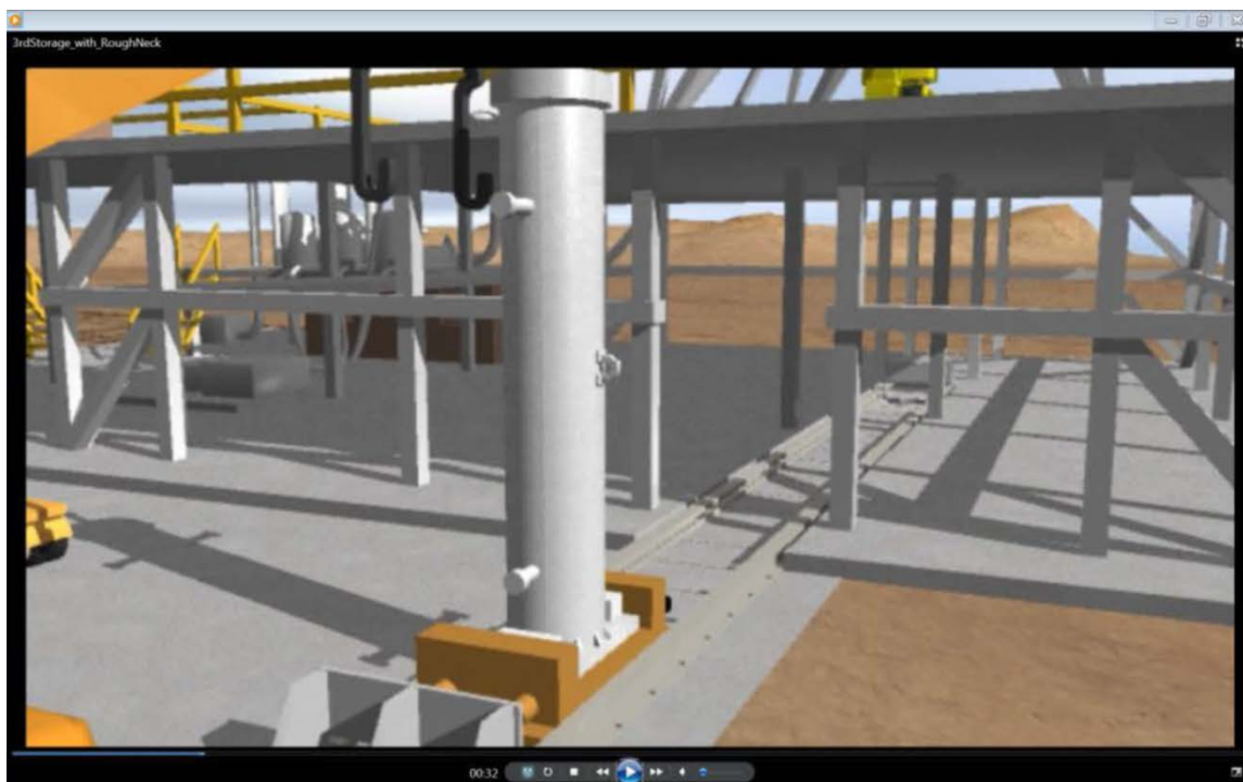
Figure 2-7. Visualization of transportation/transfer cask mounted on transfer carrier, on a track under the rig floor, leading to the well head.
