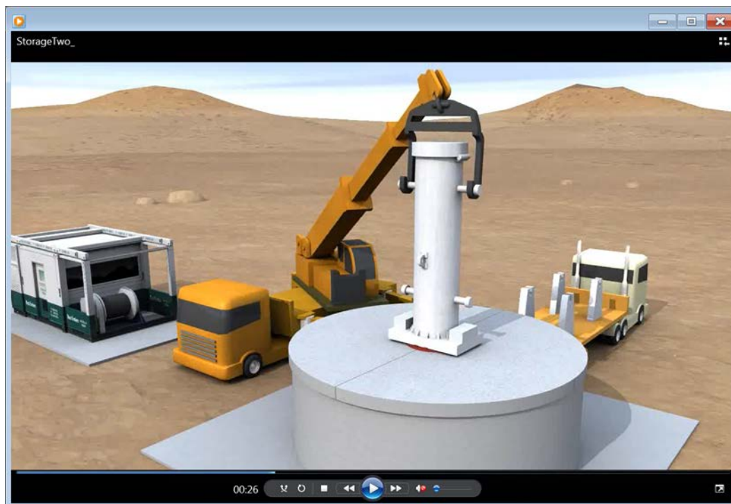
Figure 2-10. Schematic of BOP shield, top plate and shipping cask in position for waste emplacement (not to scale, and headframe not shown).
