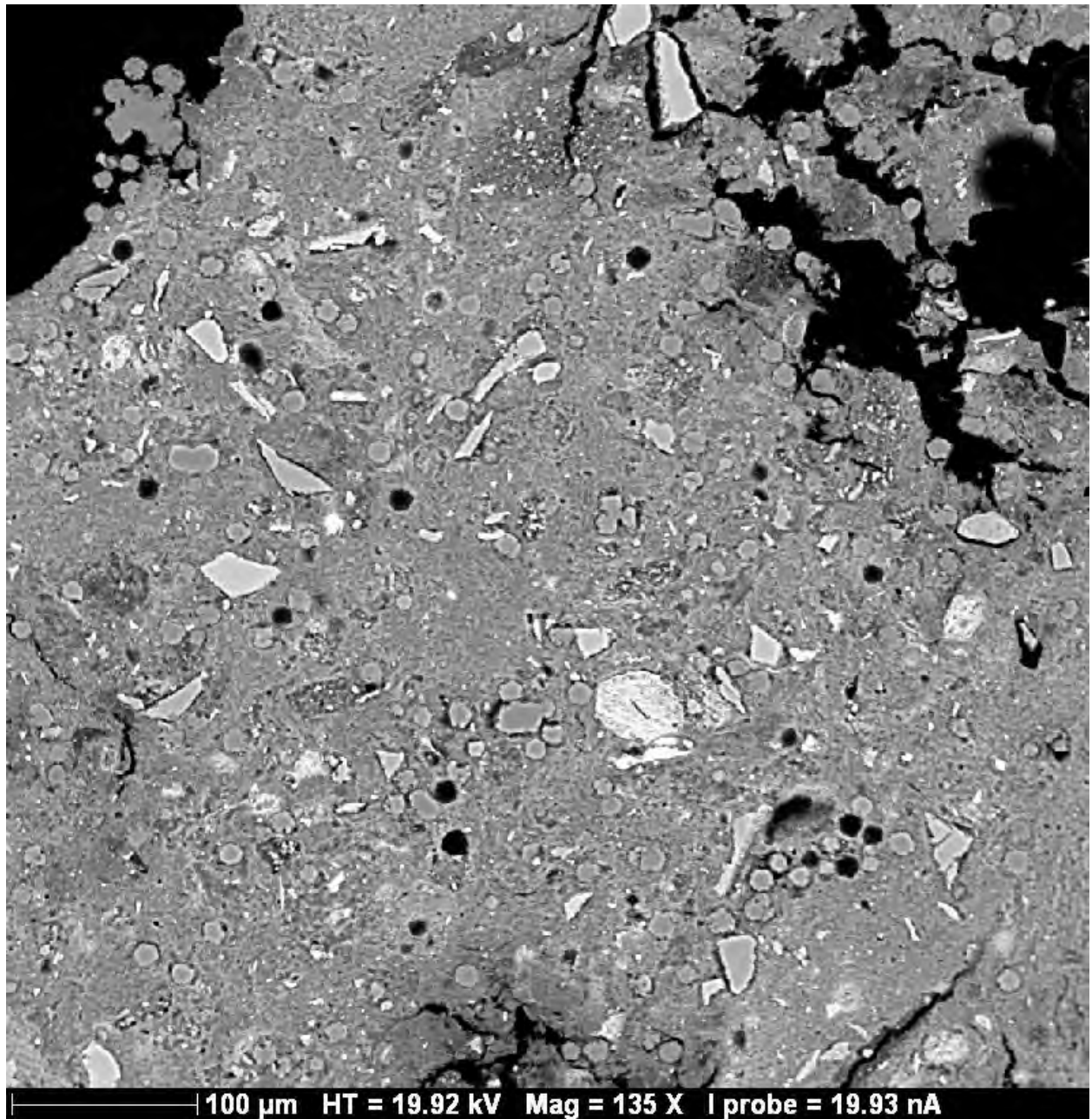
A.13-3: SEM image of EBS 13 thin section. Note analcime crystals
