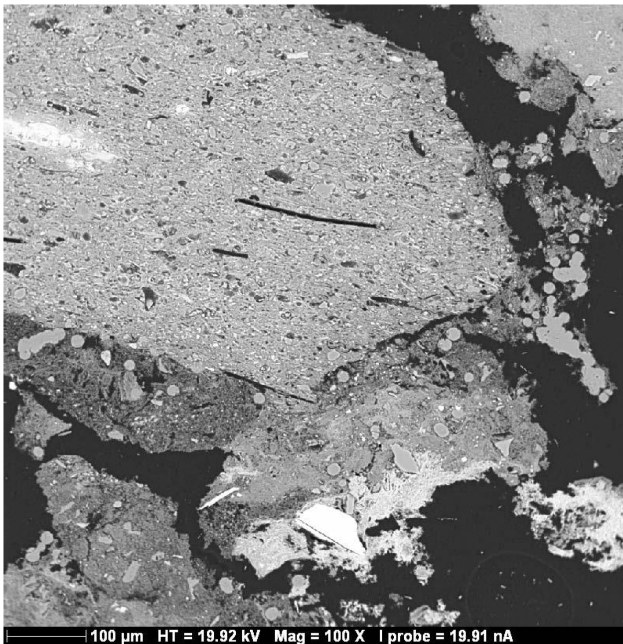
A.17-1. SEM image of Analcime ss crystals around Opalinus chunk
