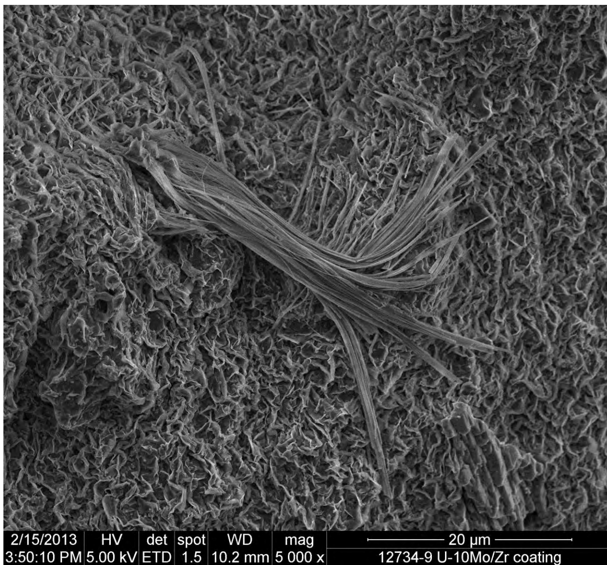
A.5-32: SEM image of illite primary spray on smectite from EBS 5
