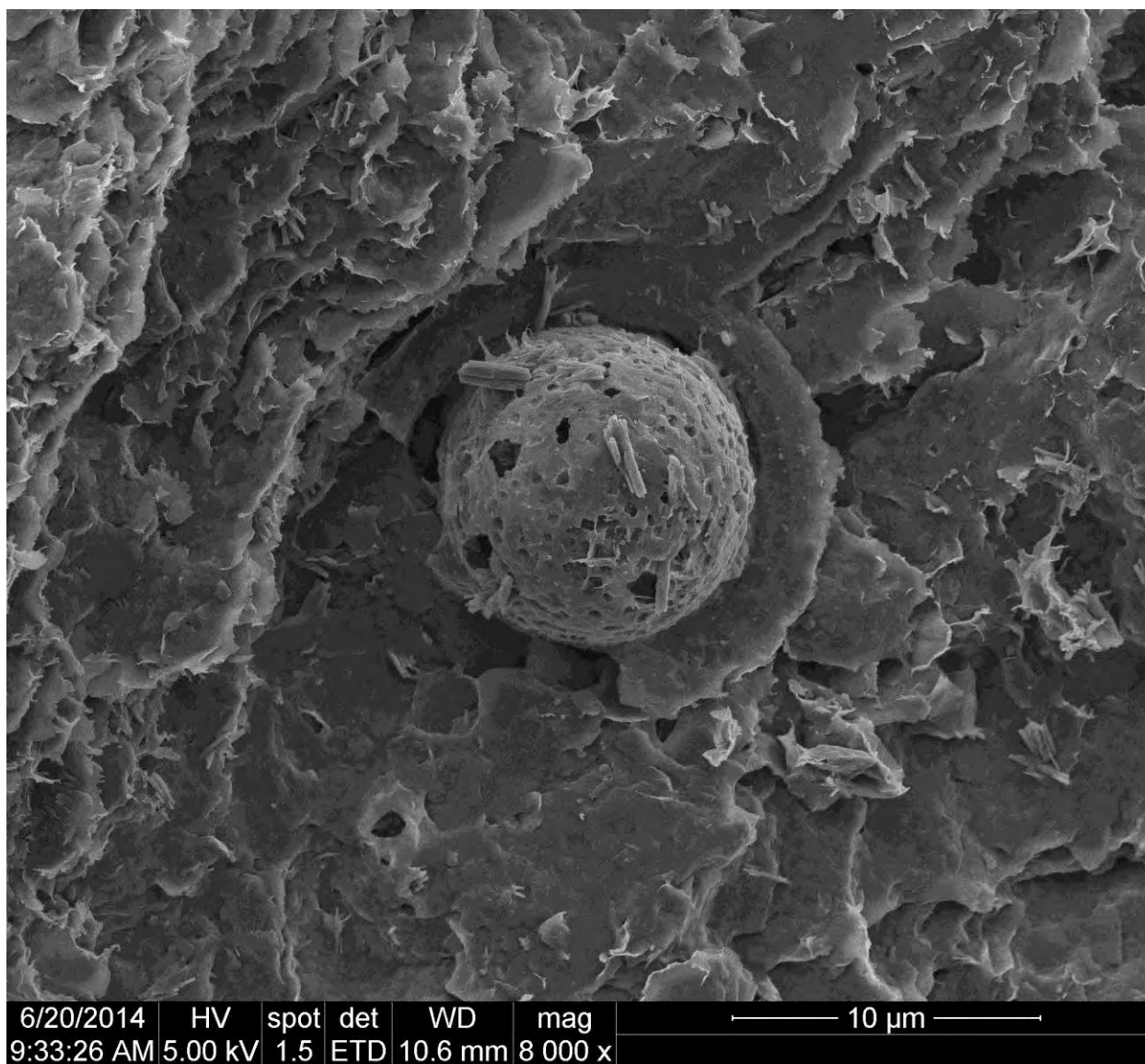
A.15-23. SEM image of calcite ball from EBS 15
