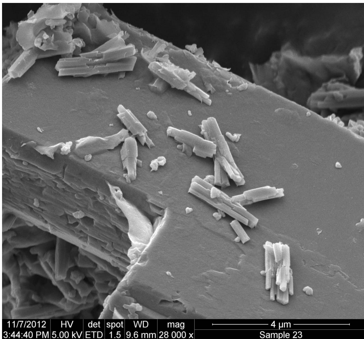
A.8-6: close up SEM image of sanidine from EBS 8
