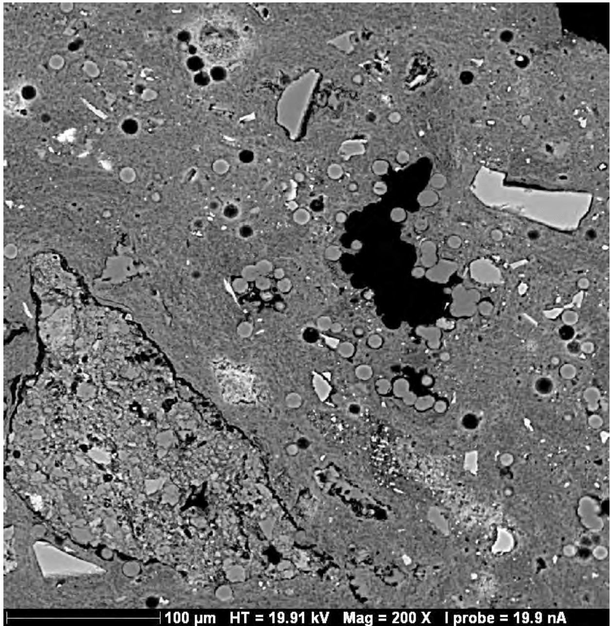
A.11-15 Backscattered Electron image of EBS-11 thin section. Note abundance of analcime (dark gray spheres with white rims) growth in both matrix and xenolith
