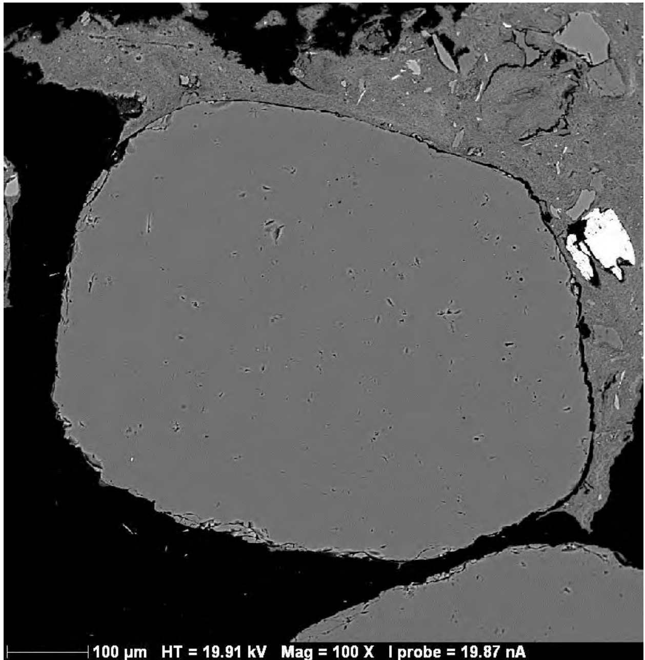
A.9-2: Back Scattered Electron image of EBS 9 thin section depicting quartz grain
