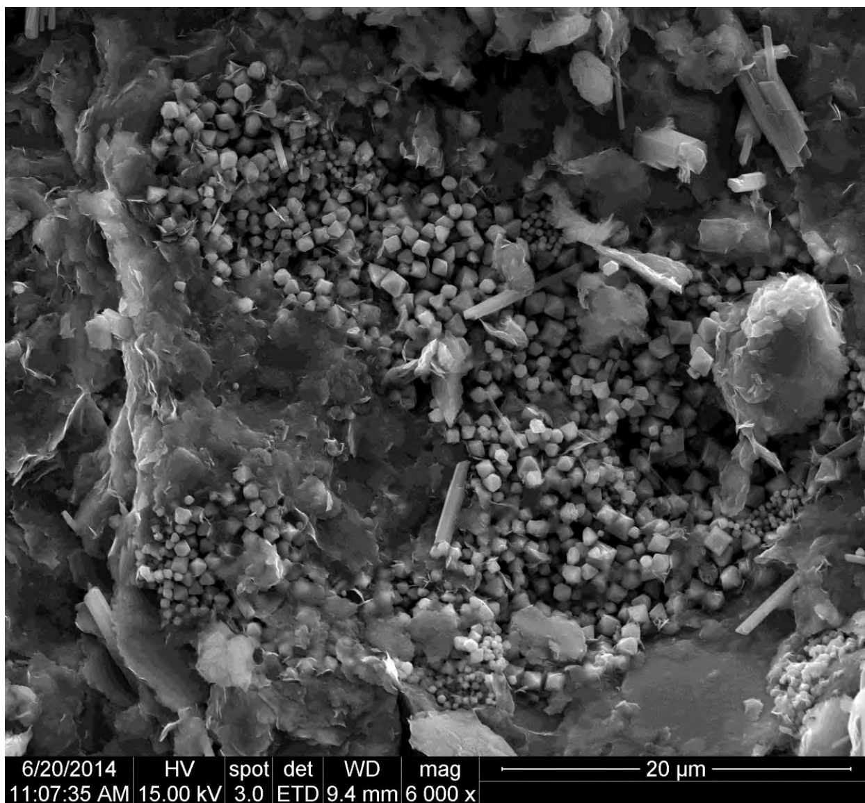
A.14-14. SEM image of pyrite framboid from EBS 14
