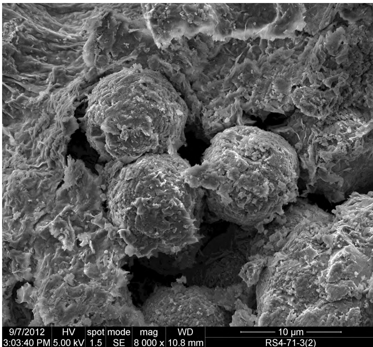
A.5-30: SEM image of Analcime replacing pumice lapilli
