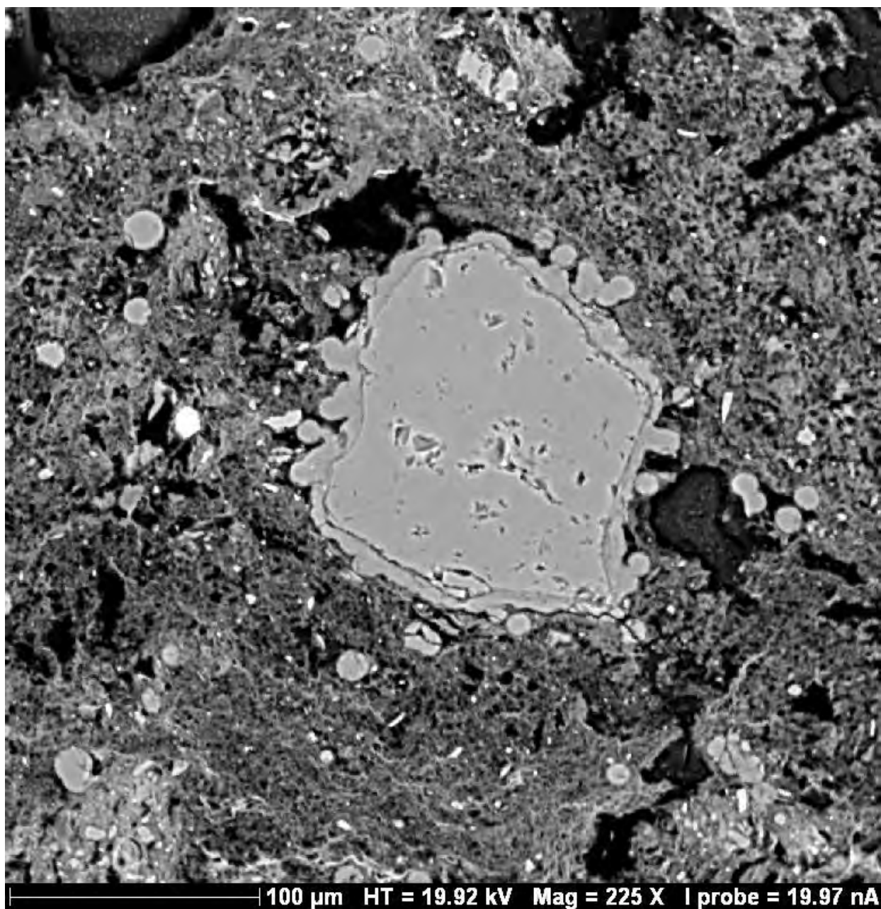
A.15-5. SEM image image of Analcime mantling plagioclase in EBS 15 thin section
