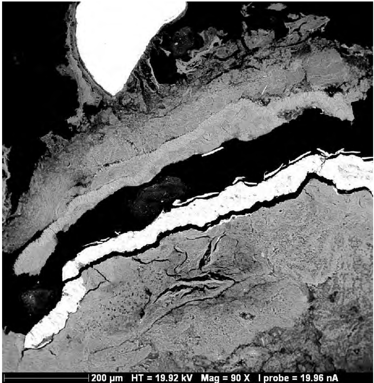
A.13-4: SEM image of EBS 13 thin section. Note Fe-phylosilicates around native iron
