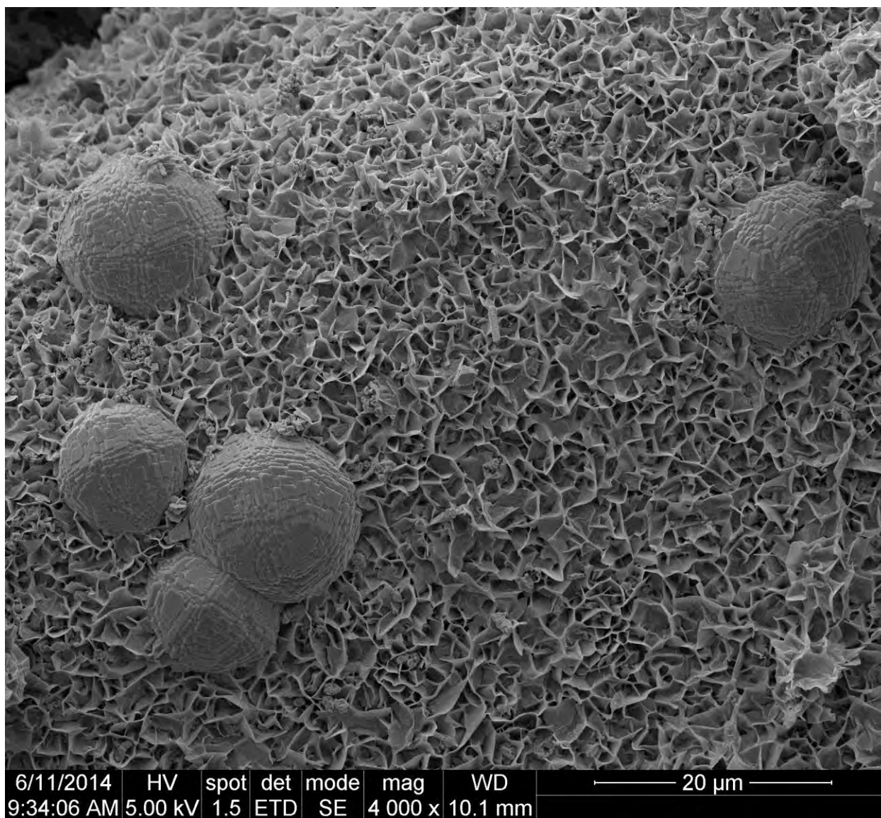
A.15-13. SEM image of Analcime-Wairakite on smectite from EBS 15
