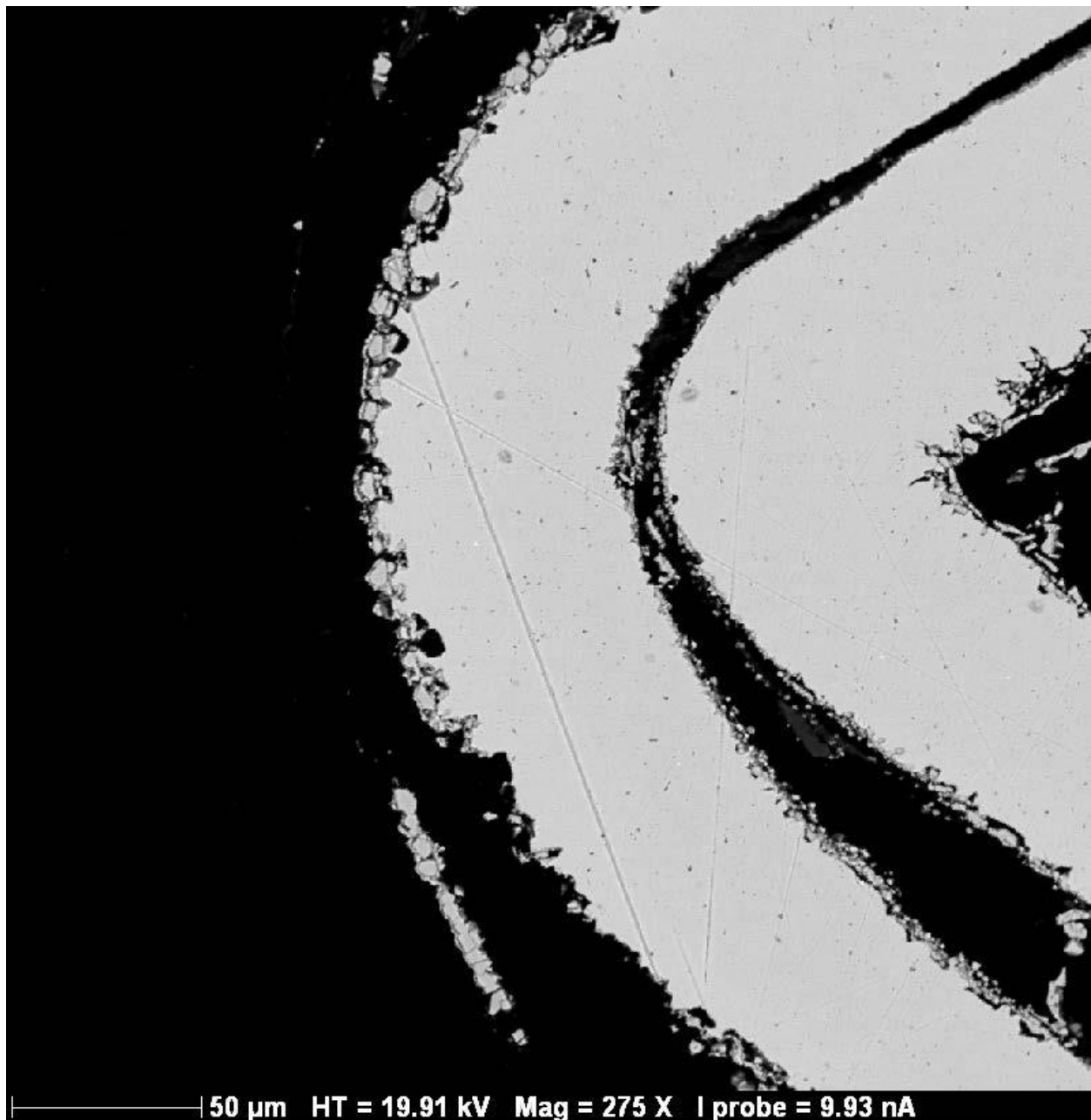
A.4-6: Back Scattered Electron image of chalcocite crystals growing over copper pit corrosion crevices
