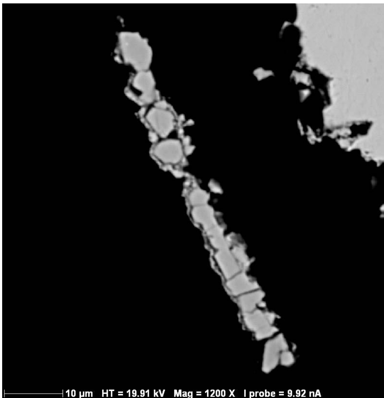
A.4-7: Back Scattered Electron image of chalcocite stringer of crystals
