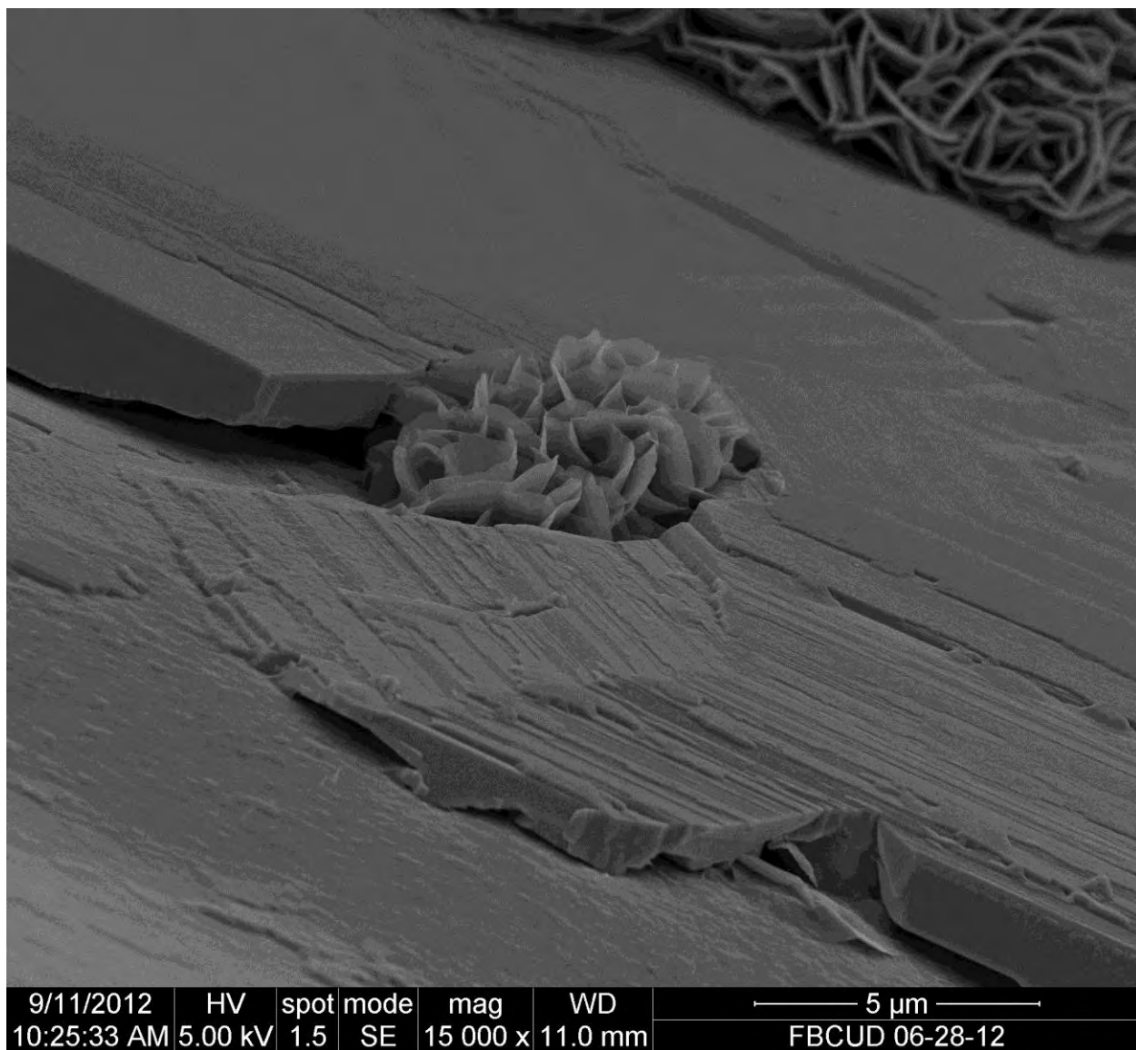
A.6-14: SEM image of iron saponite within pyrrhotite on low carbon stainless steel from EBS 6
