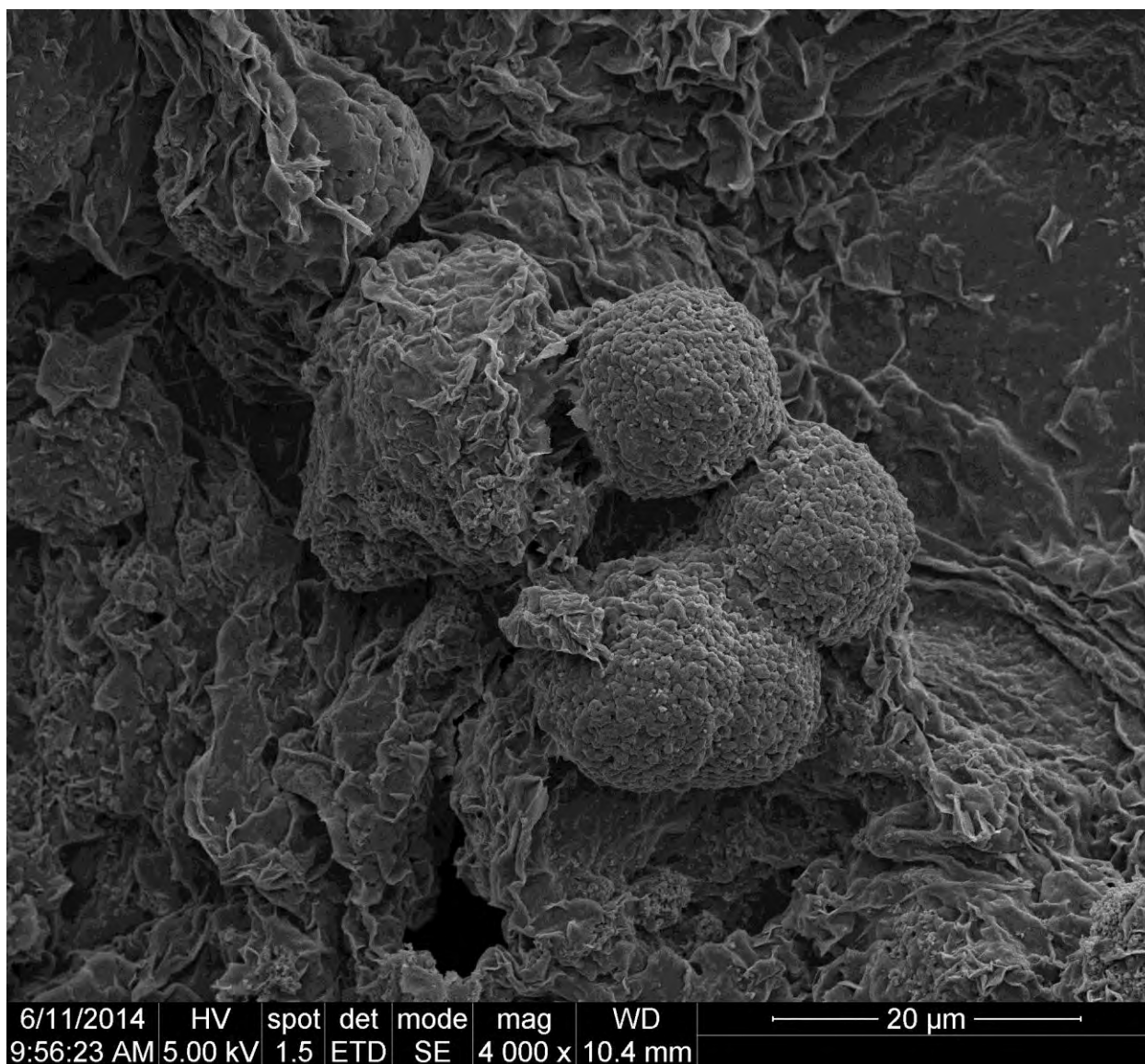
A.13-19. SEM image of smectite and Analcime from EBS 13
