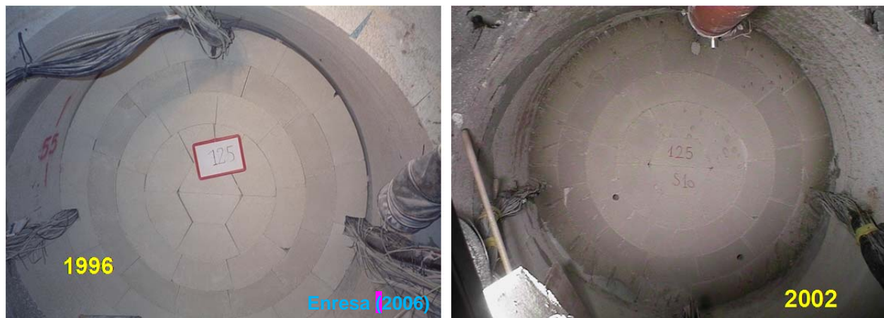
Figure 3-56. Bentonite blocks during installation of the experiment in 1996 (left) and after the first dismantling in 2002 (right). In 2002, all initial emplacement gaps between blocks were closed (from NAGRA, 2014).
