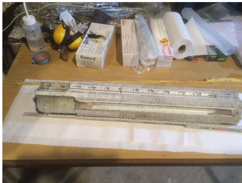
Figure 3-60. An overcore that preserves the interface between shotcrete and bentonite
