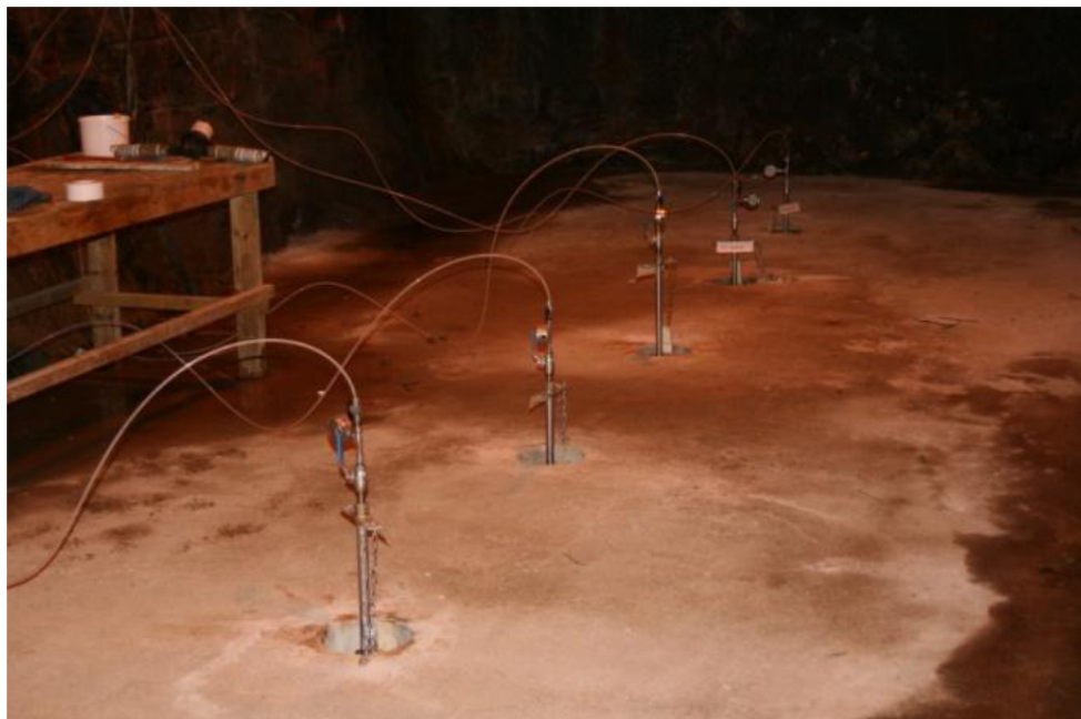
Figure 3-66. BRIE Experiment at Äspö HRL: The test niche and five boreholes (distance 1.5 m) used for initial characterization and selection of BRIE site (from SKB, 2011b)
