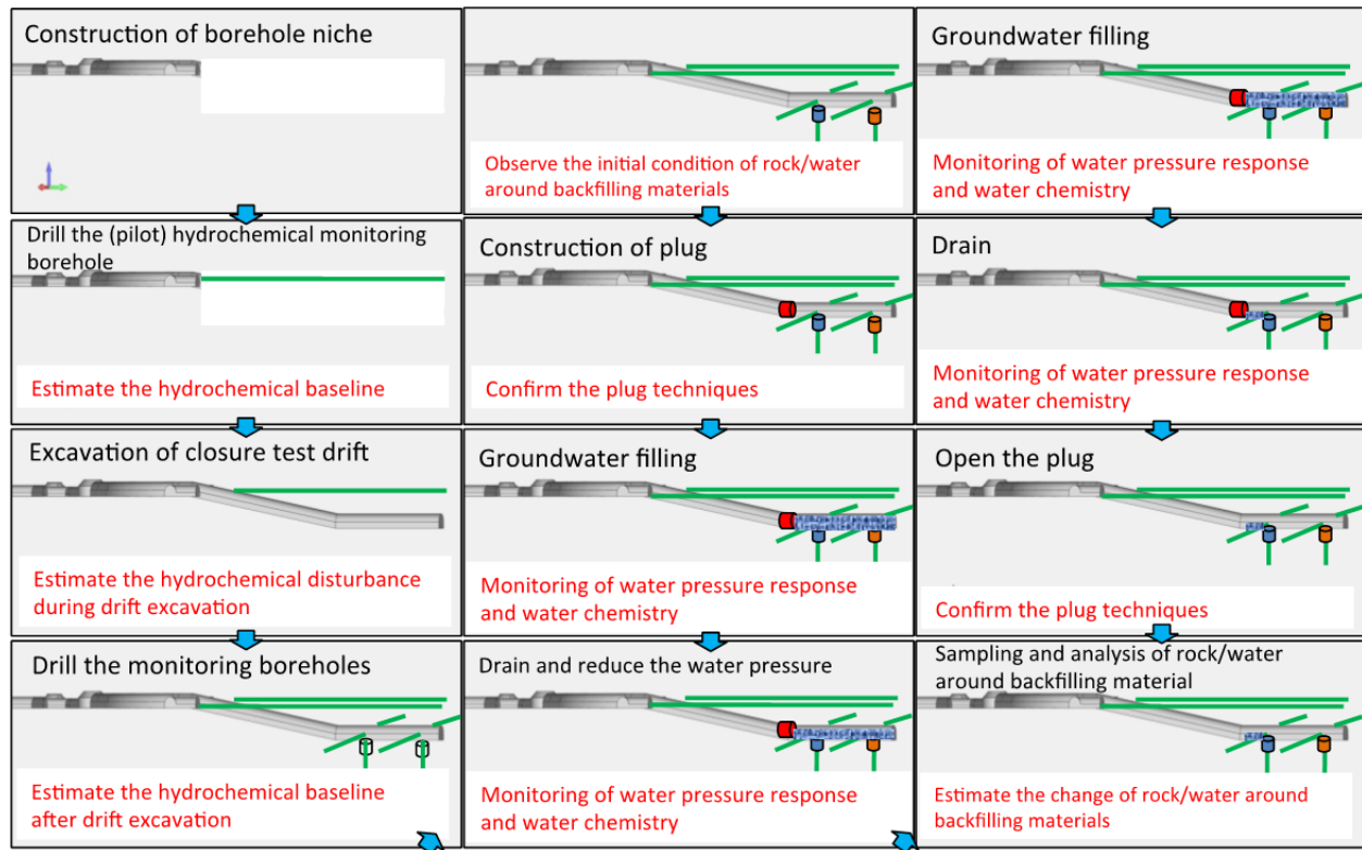
Figure 3-26. Proposed experimental sequence for GREET experiment (from Sugita, 2015)
