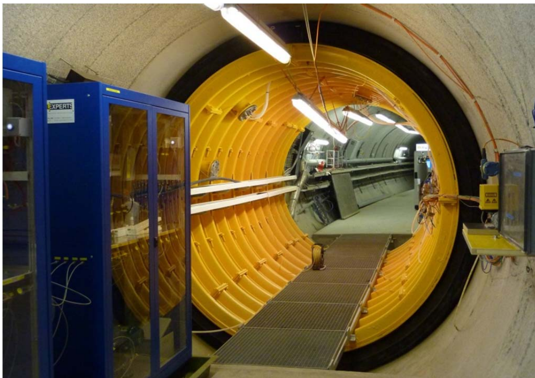
Figure 3-46. CFM field test bed at Grimsel Test Site: Tunnel packer system used to isolate the shear zone (from http://www.grimsel.com/gts-phase-vi/cfm-section/cfm-site-preparation ). Small disks with tubing issuing from them (inside yellow packer) are “surface packers” that seal the tunnel wall and collect water from inflow points. Tunnel diameter is 3.5 meters.
