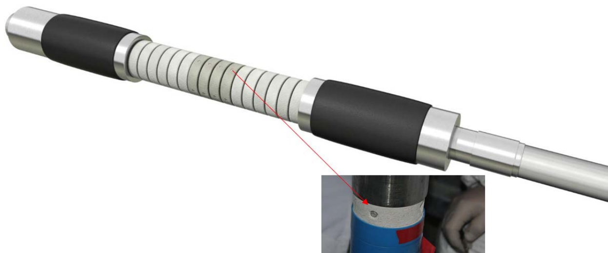
Figure 3-51. Schematic showing the LIT packer string and a photo of one of the radionuclide-doped bentonite vials after insertion into a hole in one of the four central bentonite rings
