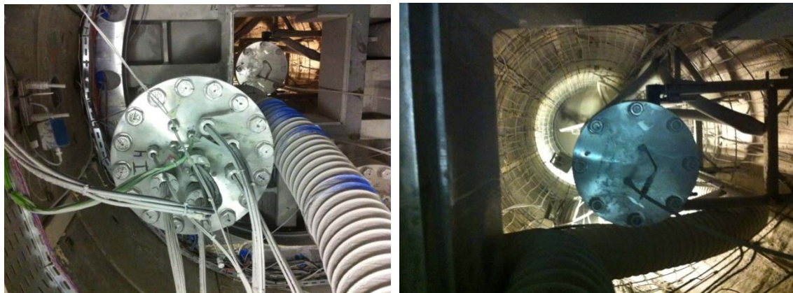
Figure 4-13. PRACLAY in situ experiment at HADES URL: Photo on left shows hydraulic seal from the outside, with an access hole to the right, which soon will be closed. Photo on right was taken from access hole into the heater gallery section, which is currently being backfilled.
