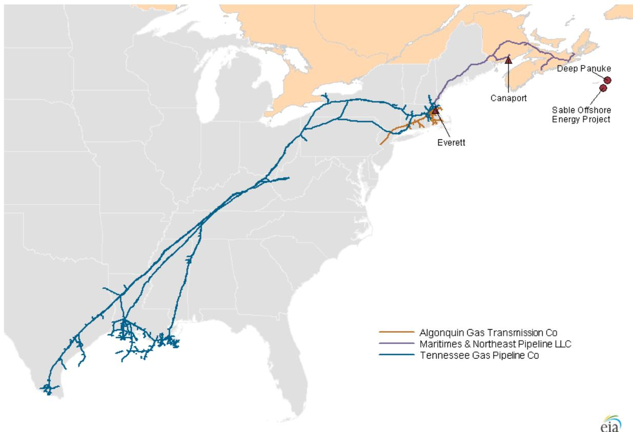
The TGP and AGT pipelines have a combined transport capacity of about 3.5 billion cubic feet (Bcf) per day delivered into New England, including gas from domestic production and storage withdrawal, Canadian production, and imported LNG. Although transport capacity is greater than average January consumption (Figure 3), peak-demand days determine the stress on the delivery system.
