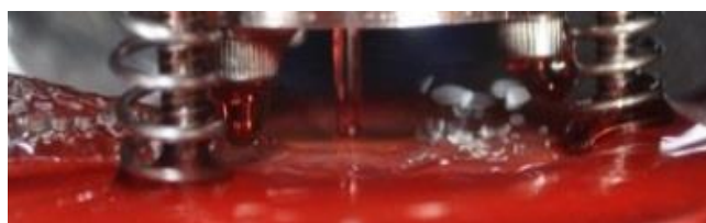
Figure 1. Results for inter-lamination thermal contact resistance (top). Picture of the test section for measurement of ATF jet heat transfer coefficient (bottom).
