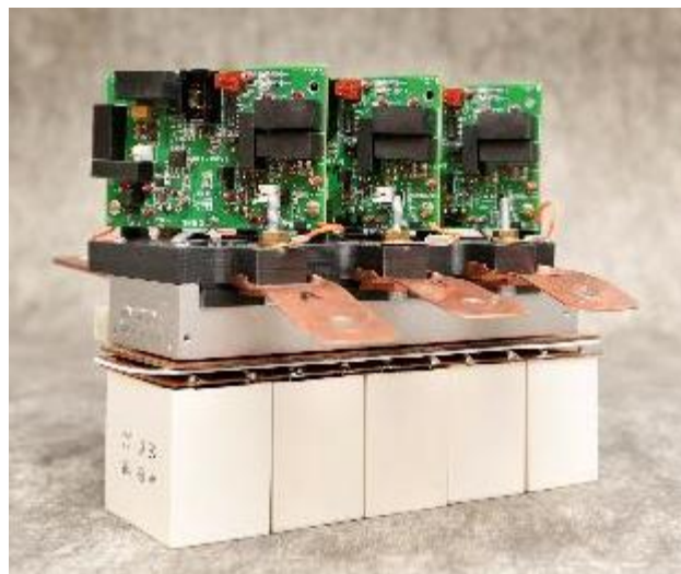
Figure 2. 10 kW SiC inverter prototype.
