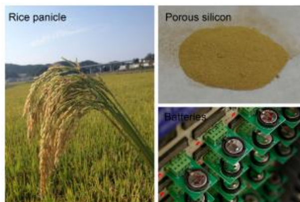
Figure 1. Photographs of rice panicle, porous silicon structures from rice husks, and lithium ion batteries with silicon anodes.
