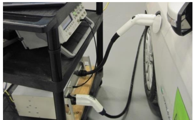
Figure 1. ANL's “man-in-the-middle” test equipment developed to test for compliance with SAE J2953 interoperability standards.
