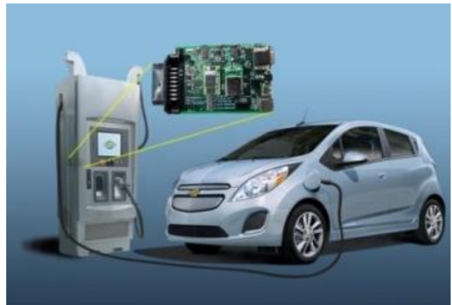
Figure 1. SpEC communication control module provides standard EVSE-PEV messaging to enable DC fast charging.
