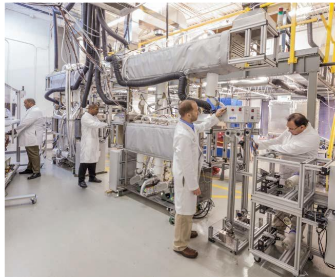
Figure 1. The one ton/year plasma oxidation oven.
