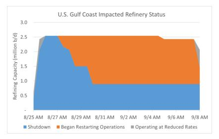
The above chart summarizes impacts to Gulf Coast refining capacity as a result of Hurricane Laura over time, as reported in D OE's Situation Reports. Impacted refining capacity is aggregated into three categories: 1) shutdown refineries (blue), 2) refineries that were shut down and have begun restarting (orange), and refineries that are operating at reduced rates (gray). Refinery statuses are updated based on various news outlets and company websites.
