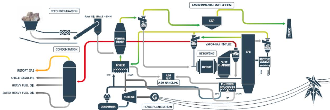
retorting technology surrounding horizontal kiln retort.<sup>53</sup> Major enhancements engineered in collaboration with the Finnish firm Outotec have increased on-stream time ~70 percent. By recovering heat from both the hot spent shale ash and flue gases and reusing it in the process, the energy efficiency of the process is significantly improved. Combustion of the residual carbon on the spent shale in a circulating fluidized bed boiler results in cleaner flue gases.
