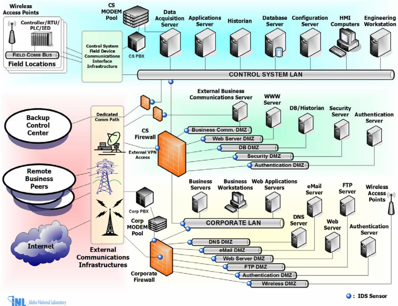
**FIG. 1 - RECOMMENDED NETWORK ARCHITECTURE - COMPARTMENTALIZING COMMUNICATION AND DEFENSE-IN-DEPTH**
