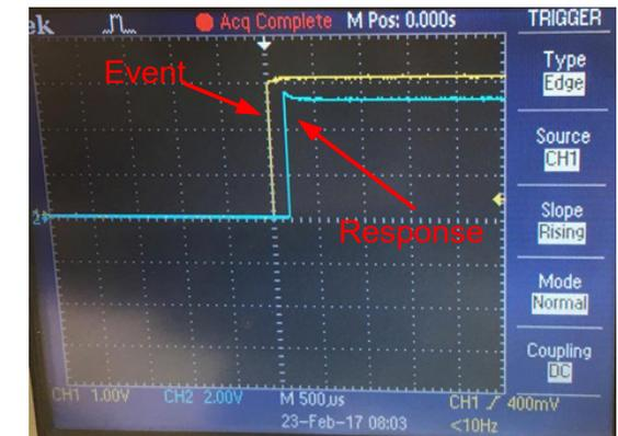
End-to-end delay time for the embedded sequence hopping implementation is **250 micro seconds**
