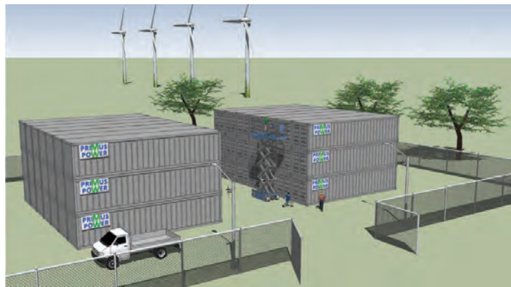
25-MEGAWATT, 3-HOUR PRIMUS POWER BATTERY PLANT; DOE FUNDING FROM THE AMERICAN RECOVERY AND REINVESTMENT ACT
