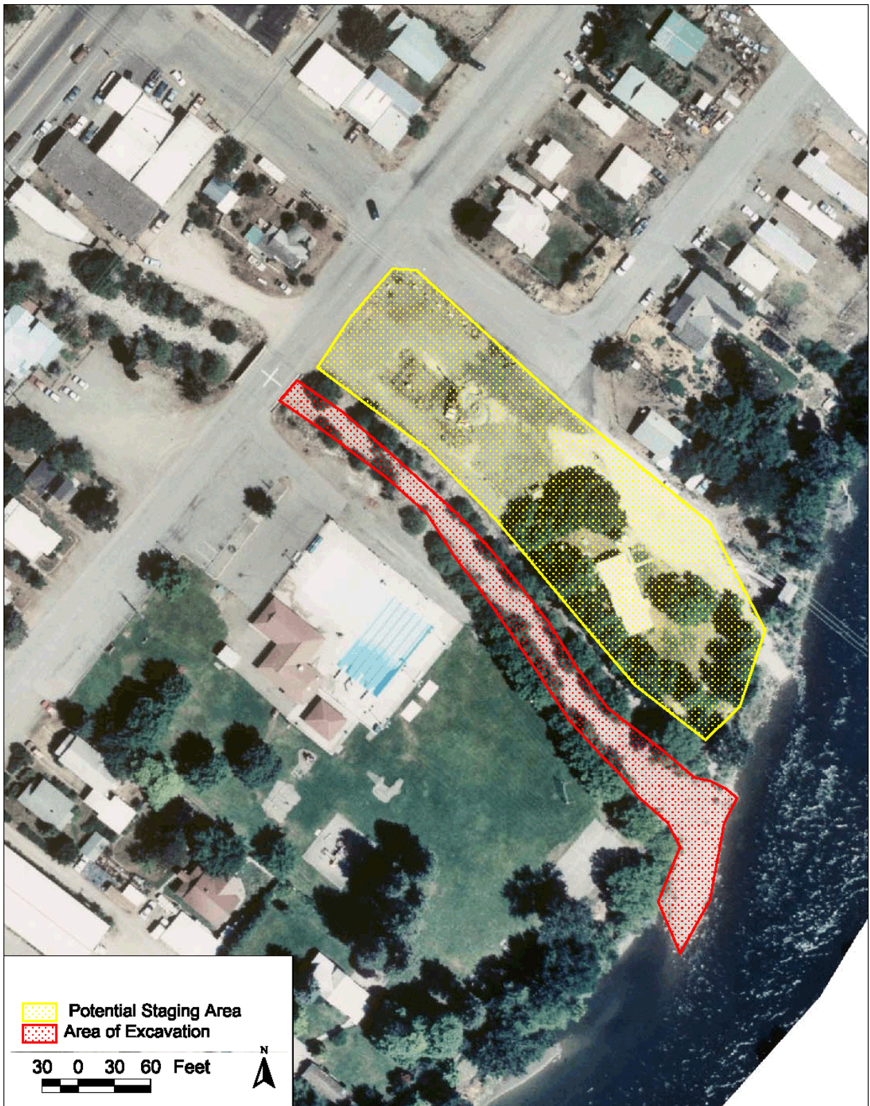
Figure 2-3. Area of Excavation of Coarse Sediment Deposition at Mouth of Salmon Creek.
