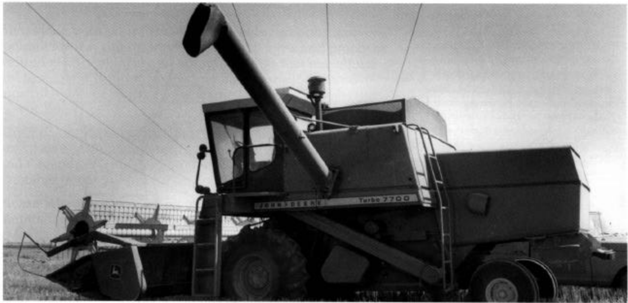
Farm equipment or open large machinery 14 feet or less in height may be operated safely under all BPA lines in cultivated fields.
