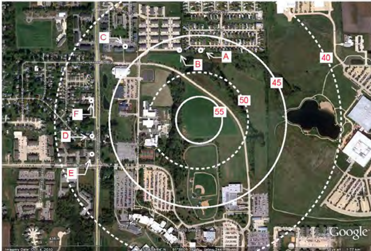
Figure 3-3. Predicted Noise Map with Rings Labeled (in dBA) [for the Clipper Liberty 2.5 MW CW99 Wind Turbine at Maximum Sound Levels]
