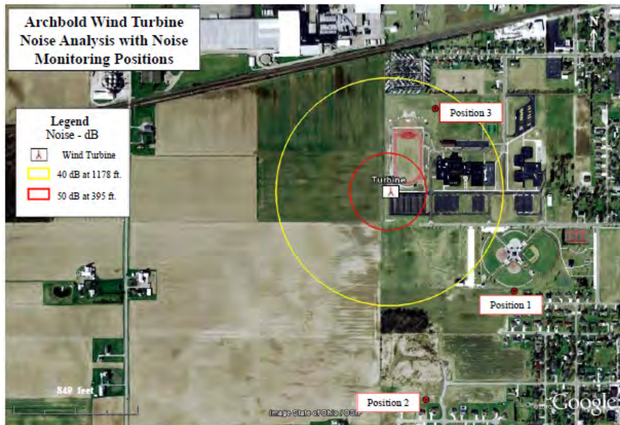
Figure 3-6. Monitoring Sites for Measuring Baseline Sound Conditions and Predicted Turbine Sound Level Contours
