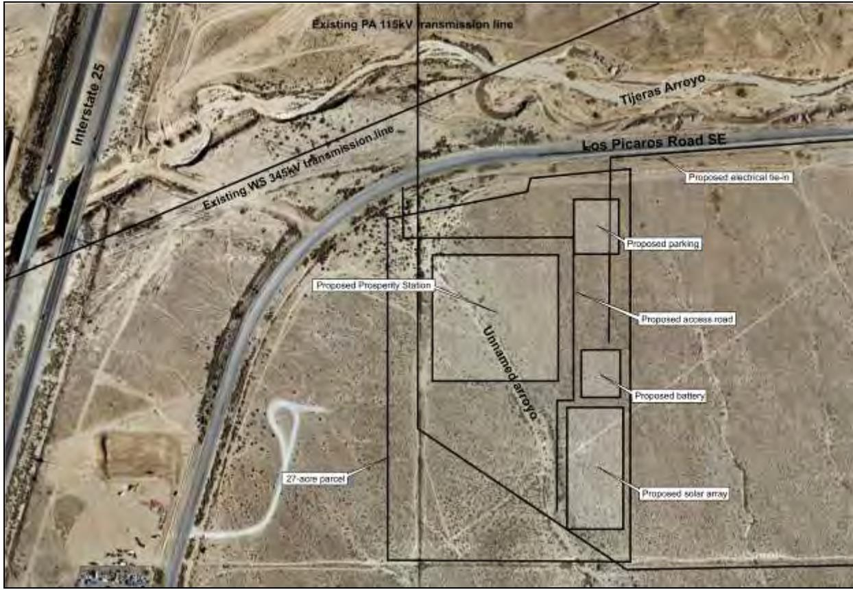
**Figure 2-3.** Site layout showing proposed facilities.
