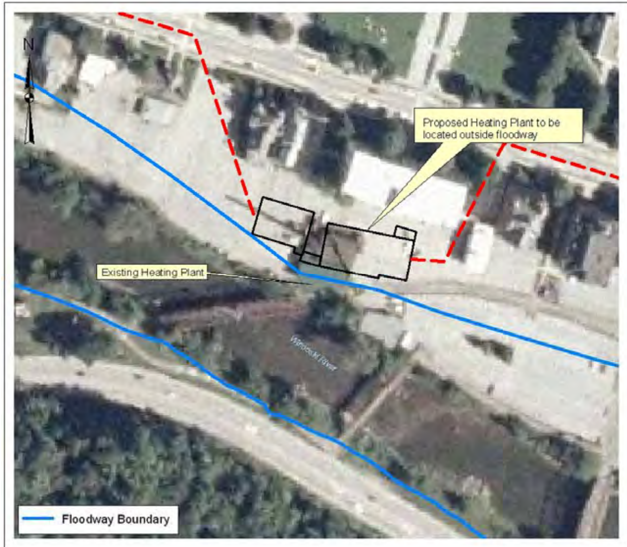
Figure 3-4. Regulated Floodway Boundary adjacent to Heating Plant
