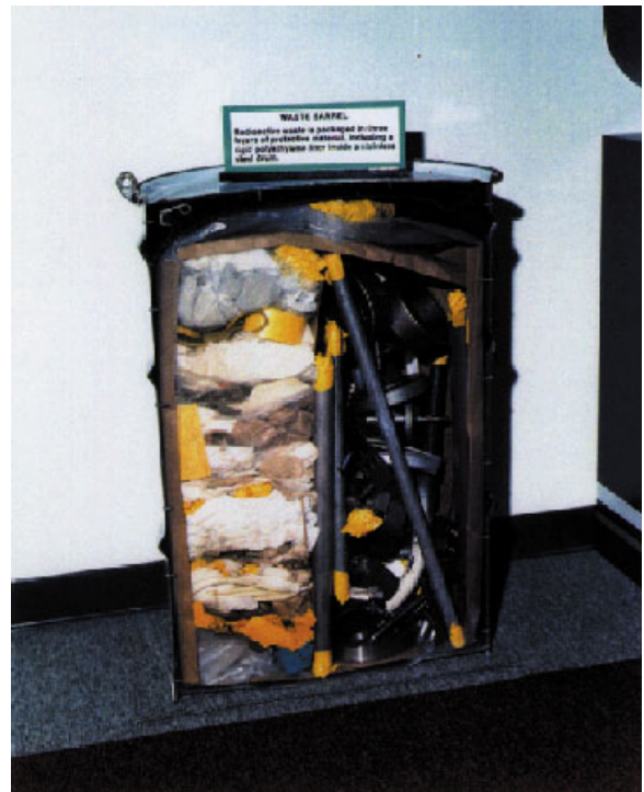
Cutaway Model of a Typical Waste Barrel
