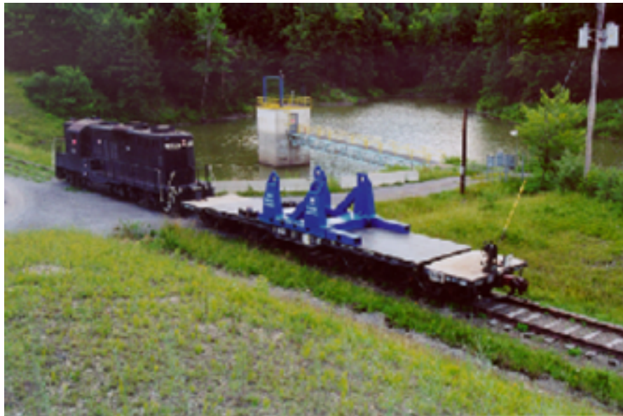
Platform for Upcoming Spent Fuel Rail Shipment
