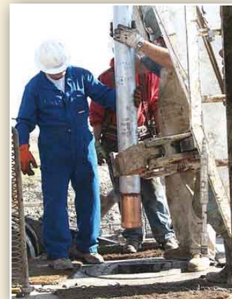
Lowering the core barrel at the PCOR Partnership lignite site.
