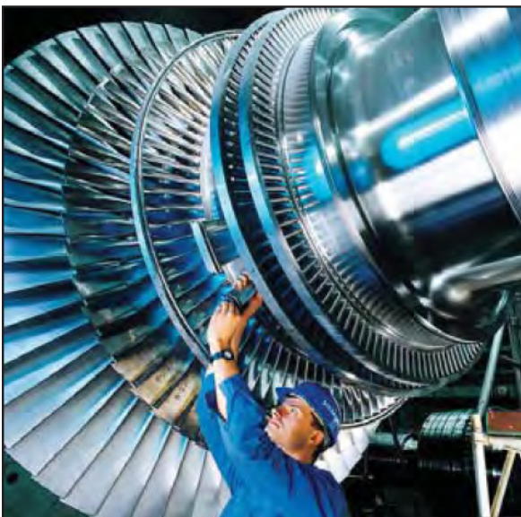
A NETL researcher inspects a steam turbine rotor assembly.
