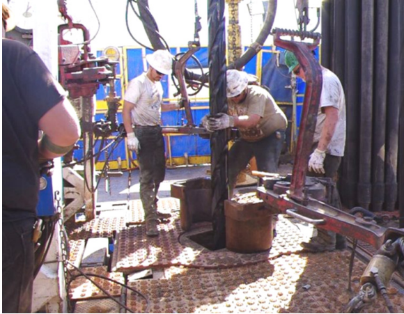
RMOTC drilling rig crew at NPR-3 (Tripping Pipe).
