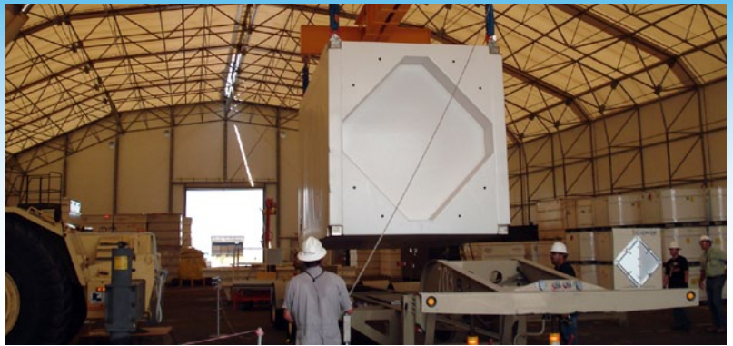
Workers remove a TRUPACT-III shipping package from a trailer for placement onto a fixed platform for loading large boxes containing legacy transuranic waste for shipment to the Waste Isolation Pilot Plant for safe, permanent disposal.
