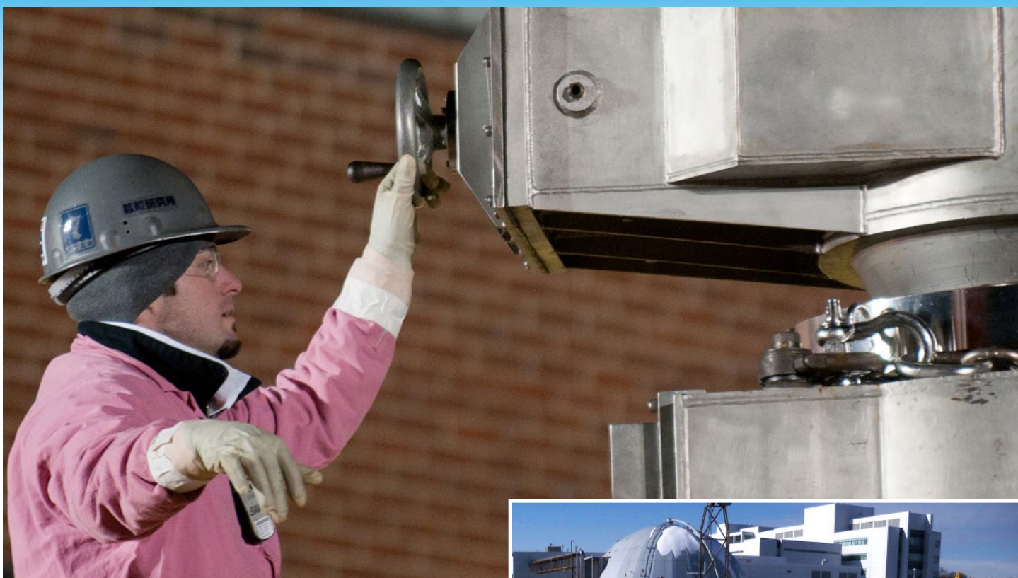
A canister of irradiated sodium-bonded nuclear fuel specimens from Argonne's Alpha Gamma Hot Cell Facility is lowered onto a shipping cask for shipment to Idaho National Laboratory.
