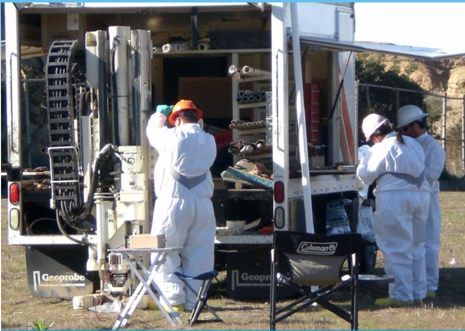
Workers perform sub-surface sampling in Santa Susana Field Laboratory Area IV.
