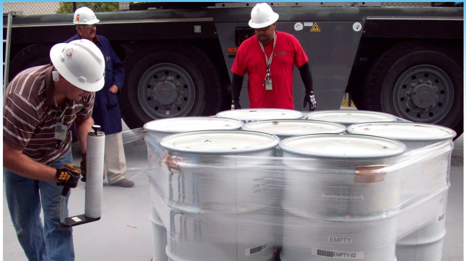
Mobile loading operators prepare drums of contact-handled transuranic waste for loading into transportation containers.
